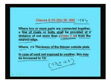
In clause 8.10.2 b of IS 800 1984 it is told that where 2 or more parts are connected together a line of rivets or bolts shall be provided at a distance of not more than 37 mm plus 40 from the nearest edge. So, this also has to be kept in mind. It should not become more than 37 mm plus 40 where t is the thickness of the plate thickness of the thinner plate. So, where t is the thickness of the thinner outside plate in case of work not exposed
