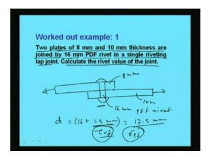
Now, the some of the worked out example if we go through then we will be able to understand how to calculate the strength of a joint. If we go through 1 or 2 worked out example then we will be able to understand. One example has been given here that is 2 plates of 8 mm and 10 mm thickness are joined by 16 mm power driven filled rivets. This PDF means power driven filled rivets in a single riveting lap joint calculate the rivet value of the joint.
