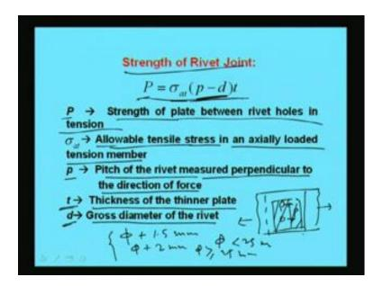
So, how do we find out the strength of the rivet joint from this. That strength will become the sigma at into p minus d into t. What is capital P? Capital P is the strength of plate between rivet holes in tension right. Strength of plate between rivet hole in tension. So, here the strength we will find out right? Now, if pitch is P then p minus d per pitch
