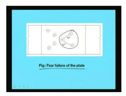
So, another chances of failure will be like this tear in failure may when it is zig-zag that also it may fail which is very unlikely the tearing may happen like this. Though it is very unlikely this type of failure also may come into picture.
