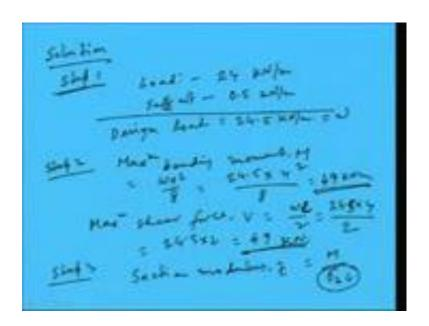
So, let us assume say 165 is the maximum say let us assume, sigma be the permissible compressive stress in bending say 110 Newton per millimeter square. Therefore, the Z the section modulus will become M by sigma be that is 49 kilo Newton meter. If I make into Newton millimeter, this will be into 10 to the 6 and sigma be is say we have consider 110 MPa.
