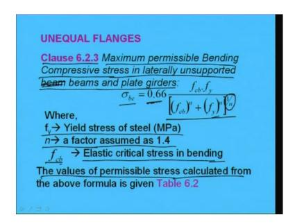
So, in clause 6.2.3 it is described that the Maximum permissible Bending Compressive stress in laterally unsupported beam and plate girders can be written as: sigma bc is equal to 0.66 into fcb into fyy fcb to the power n plus fy to the power n whole to the power 1 by n right. This is given in the clause you can just refer to clause where it is explicitly defined.
