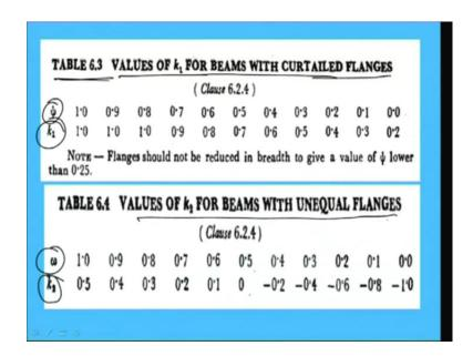
Now, as was telling you that in table it is given like in table 6.3 values of k1 for beams with curtailed flanges has been given. So, for different psi you can find out values of k1 and similarly, for different omega you can find out the values of k2. So, values of k2 for beams with unequal flanges. So, from this we can find out values of k1 and k1 from table 6.3 and 6.4.
