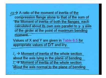
Now what it omega? Omega is a ratio of the moment of inertia of the compression flange alone to that of the sum of the moment of inertia of both the flanges, each calculated about its own axis parallel to y-y axis of the girder at the point of maximum bending moment. Values of X and Y are given in table 6.5 for appropriate values of D by T and I by ry right.
