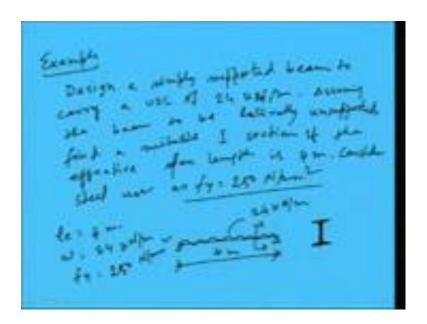
So, example is like this say design a simply supported beam to carry a UDL of say 24 kilo Newton per meter. Assuming the beam to be laterally unsupported find a suitable say I am telling I section let us do for I section if the effective span length is 4 meter. Consider steel used as fy 250, so fy value is 250, let us consider. So, what we are seeing
