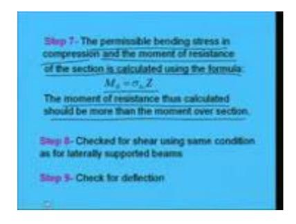
Next step is step 8, so once we find out a suitable section from bending moment point of view, then we can go for checking of shear. How do we make checks here? As we have done in case of earlier; that means, we will find out what is the maximum shear then we can find out average shear stress; what is developing and the allowable shear stress, whether it is less than that or not we have to check and accordingly we have to act right.
