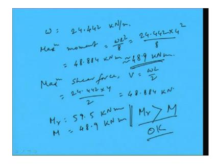
So, actual load will become 24 plus 0.442 means 24 442 kilo Newton per meter right. So, now we can find out the maximum moment right that will be wL square by 8, w is 24.442 into 1 is 4 by 8, so this is find out 48.884 kilo Newton meter or say I can write
