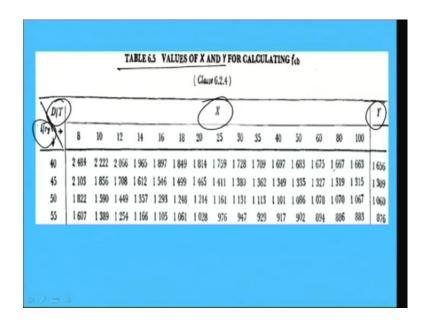
And in table 6.5 directly we can find out value of X and Y with the values of D by T and 1 by ry. Otherwise, those you are going to develop the software develop the programming
