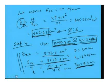
This is 8603.6 centimeter cube, so those things we will provide here right. So, 8603.6 this is centimeter it was centimeter to the 4. So, we are making millimeter to make in centimeter. So, if we calculate we are going to get 4.735 millimeter this is less than delta allowable which is 12.33 millimeter; that means, from deflection point of view this is ok.
