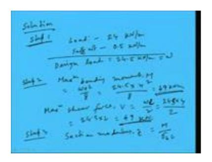
So, when we go for the solution say step 1, we will try to follow the steps which we have discussed earlier. In earlier in design procedure we have told step 1 step 2 step 3 like this we have made. So, for the sake of simplicity same steps I am going to follow 1 by 1 then you can have a systematic way to design the whole thing right. So, in step 1 what it is told that that we have to find out the load acting on the beam.
