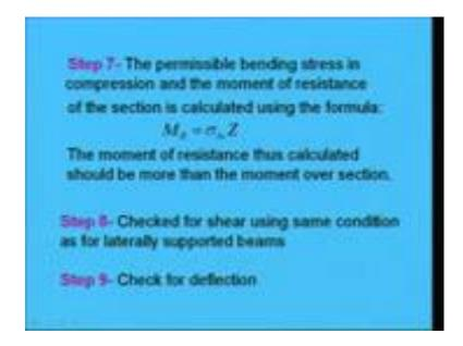
So, step 7 what we will do that the permissible bending stress in compression and the moment of resistance of the section is calculated using formula: MR is equal to sigma be into Z, where the moment of resistance is calculated it should be more than the moment over the section. So, in this way we can find out the moment of resistance which is sigma be into Z, where Z is the section modulus.
