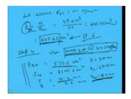
Another is we have used the beam this say ISMB 300 at 44.2 kg per meter that means, if I make Newton this will be 44.2 Newton per meter; that means, 0.442 kilo Newton per meter. So, self weight will be 0.442 kilo Newton per meter right. And load, impose load is 24 kilo Newton per meter.
