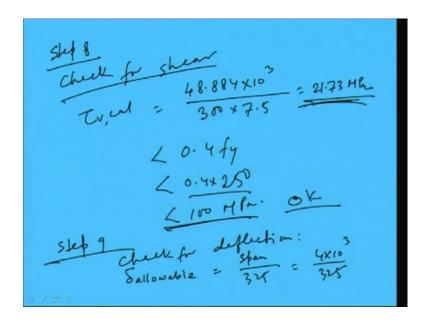
Next what we will do next is step 8; that means, check for shear right. Check for shear means, we know tau v say calculated will be maximum shear was 48.884 and this is kilo Newton. So, I am making Newton and by d into tw, so d is 300 and tw is 7.5, so this is coming 21.73 MPa right. So, shear stress developing is 21.73 MPa and it has to be less than 0.4 fy and this 0.4 fy is 250, so if we multiply 0.4 into 250 this is becoming 100.
