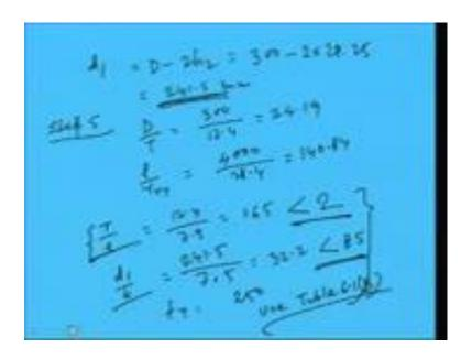
So, for D by T 24.19 and l by ry 140.84 and fy is 250 we can find out the value of sigma bc. So, by interpolation we can finally, find out 103.71 MPa Now, it is not very easy to find out the sigma bc value from table we have to make interpolation linearly interpolation. So, if you check at your own when you will do you see for this ratio and this ratio you will get sigma bc value as this right.
