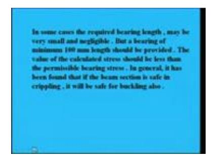
Again whatever we are calculating the bearing length, that may be negligible or very small. Sometimes it may be very small means; in some cases the required bearing length may be very small and negligible. But in this case, a bearing of minimum 100 mm length should be provided. So, in any case we should provide a minimum of 100 mm length of bearing should be provided.
