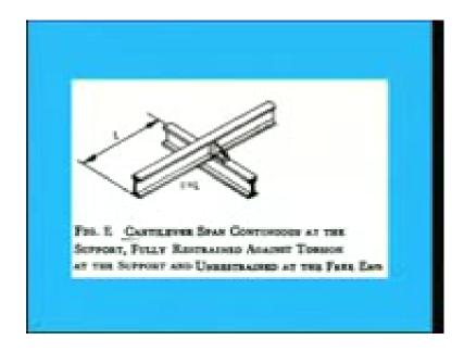
Cantilever span continuous at the support, fully restrained against torsion at the support and unrestrained at the free end. In this case effective length will become equal to 1. So, these are the some conditions where Codal provision has been given and through that, we have to find out the effective length for calculating the sigma bc.
