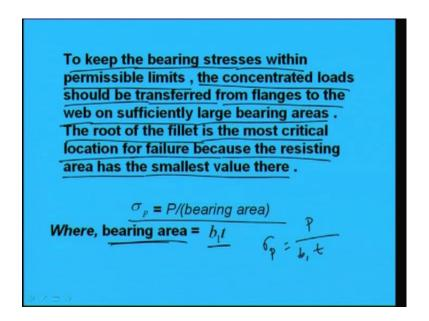
So, to keep the bearing stresses within permissible limits, the concentrated load should be transferred from flanges to the web on sufficiently large bearing areas. The root of the fillet is the most critical location for failure, because the resisting area has the smallest value there. As the resisting area is becoming less, so chances of failure will be there.
