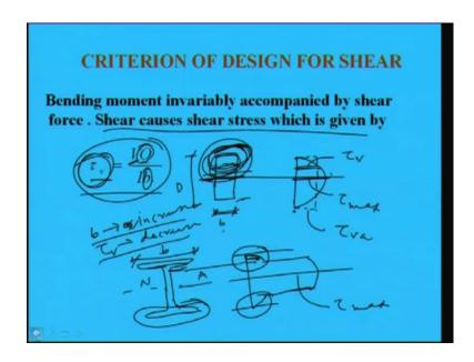
Now, we will discuss about some criteria to find out the shear stress and the design value of the shear stress right. As I told that first step is to find out the appropriate section of the beam from the bending stress point of view. Now, what we will do we will try to find out the what is the shear stress developing for that particular section and what is the allowable stress allowable shear stress of that section.
