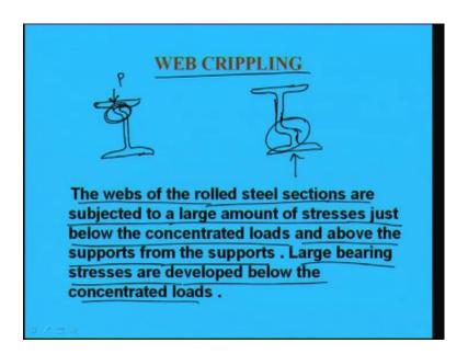
Another important aspect of the design of beam has is, the web crippling means we have to see whether the beam whatever we have designed is safe against the crippling effect or not. So, what is the web crippling let us see first that if say suppose say concentrated load
