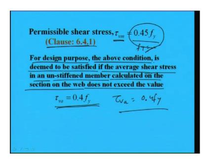
Suppose we are computing the shear stress suppose here;, so first moment of the outer area, so from here we can find out right. So, in this way Q value can be find out. Now, you see the moment you are increasing the value of means, where value of Q then tau v will be increasing; that means, if you go below from the extreme fibre or go up from the extreme bottom fibre then this area will become more.
