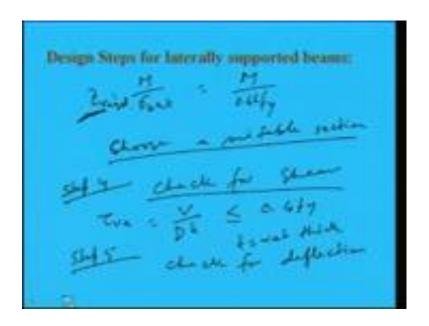
So, as we know in last class we have shown check for deflection means, we have to see what are deflection is coming that should not be greater than span by 325. That means, le by 2 3 25 span means effective length by 325. So, the calculated delta deflection should not be greater than this that we have to check. So, how do we calculate the delta?
