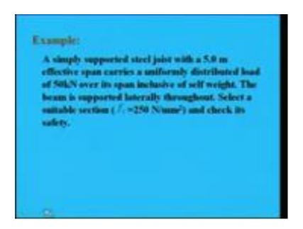
Now, we will go through 1 example, today I will give the example means I will write down the example here; you try to do at your own time and in next class I will solve the problem and we will see whether it is matching with your workout example or not. A simply supported steel joist with a 5 meter effective span carries a uniformly distributed load of 50 kilo Newton over its span inclusive of self weight right, 50 kilometer per meter over a span inclusive this.
