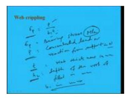
Now, here we can say that sigma P which we are going to develop P by b1 into t. So, sigma P we can write that bearing stress right. And say this can be find out in MPa, if P is the concentrated load or reaction in case of support it will be reaction from support in Newton right. And then b1 we have now, t t is the web thickness in millimeter. So, this is Newton and this is millimeter, this is millimeter.
