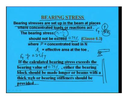
Another aspect is the bearing stress; bearing stress where it develops as we know where the concentrated load is there or where the support is there suppose simply support is there. So, the stress will develop here some, because of concentrating force in nature the stress will develop. So, bearing stresses are set up in the beam at places where concentrated loads or reactions act right.
