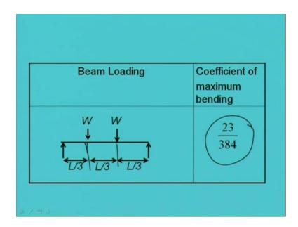
So, these are some standard conditions we are showing which you can remember like, if the load is at 1 third 1 third distance then the coefficient will become 23 by 384, right.
