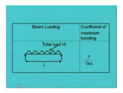
For some standard loading condition and boundary condition we know what are the deflection coefficients right. Like say suppose we have a simply supported beam with
