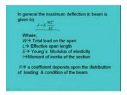
Now, here whatever equations we have written we know that W is basically the total load on the span, not UDL load the total load on the span. And L is the effective length of the beam and E is the Young modulus of elasticity and I is moment inertia of the section. And K is the coefficient depends upon the distribution of the loading and end condition of the beam. So, with this we can find out the maximum deflection right.
