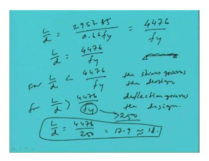
So, L by d will become 2953.85 by sigma be means 0.66 fy. So, this will lead to this equation the 4476 by fy. So, for this particular case L by d is becoming 4476 by fy. So, we can limit the values in this way right, which case we are going to limit that is the simply supported beam having UDL load, right.
