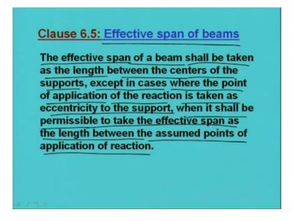
And in clause 6.5 the effective span of beams have been defined. That is the effective span of a beam shall be taken as the length between the centers of the supports, except in cases where the point of application of the reaction is taken as eccentricity to the support, when it shall be permissible to take the effective span as the length between the assumed point of application of reactions. These are told in clause 6.5 regarding effective span of beams 5 minutes more no.
