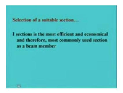
And it is also observed that the section of I section is the most efficient and economical and therefore, most commonly used section as a beam member. So, we will see mostly we are using I section as a beam member, because that will make most economical why. As we told that if a section is like this say rectangular section then what will happen. We know that, this is the stress diagram and we know that sigma is basically M by I into y.
