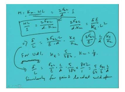
Again we know M is equal to Km into WL, so if we put the value this will become 2 sigma by d into I right. So, M is equal to we can write Km into WL and earlier we found M is equal to this is 2 sigma bc by I right. So, I can write WL by I will become 2 sigma bc by d into Km from these 2 equations I can write like this. So, WI by WL by I is equal to 2 sigma bc by d into Km right.
