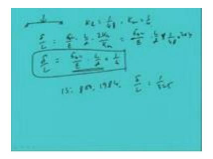
That means, if we have a simply supported beam if we have a point load then we know KL is 1 by 48 and Km is 1 by 4. So, in this case delta by L will become say sigma by E into L by d into 2KL by Km. So, if we put the value the sigma bc sigma bc by E into L by d into this will become 1 by 48 and 2 into 4. So, this is finally it becoming sigma bc by E into L by d into 1 by 6.
