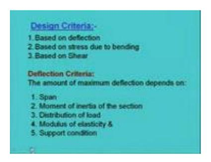
Now, design criteria. So, as I was telling the design criteria will be based on what type of failure we are going to have for the member. As we showed the failure is coming because of bending, because of shear and because of deflection. So, design criteria also will be based on deflection and bending then shear. So, 3 things we have to see that we will design the beam member with basically 3 conditions: one is deflection, another is bending and another is shear.
