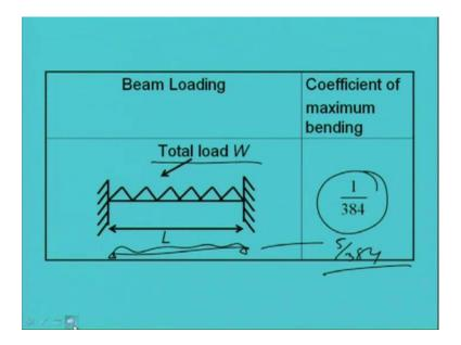
Again if beam is fixed end with fixed end at 2 side and which are UDL load then this will become 1 by 384. If you remember if it is simply supported with UDL load then this is 5 by 384. So, in this way we can find out the maximum deflection.
