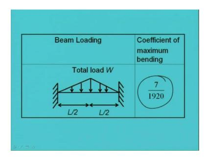
And if beam loading is triangular like things then the deflection coefficient will come say 7 by 1920 right. If the load is at the midpoint with beam end condition as fixed then the coefficient will become 1 by 192.
