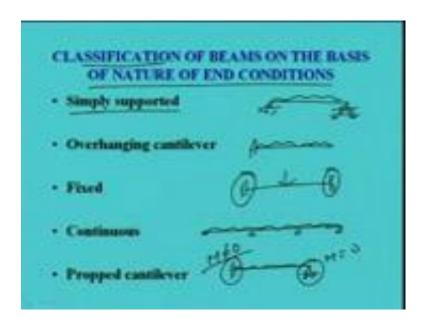
Now, this beam members can be classified into different way as per the nature of end condition right: one is say simply supported we can say simply supported beam; that means, as per the boundary conditions of the beam member we can classify the beams into this categories like simply supported this is called simply supported say, suppose loading is say UDL loading or something is there.
