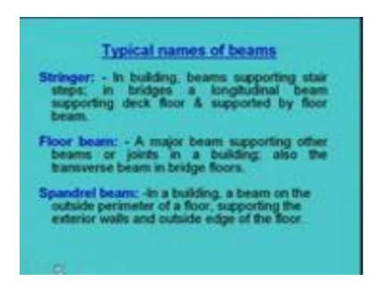
Next is Stringer: in building, beam supporting stair steps, in bridges a longitudinal beam supporting deck floor and supported by floor beam this type of beams are called Stringer. And another name we use is floor beam: a major beam supporting other beams or joints
