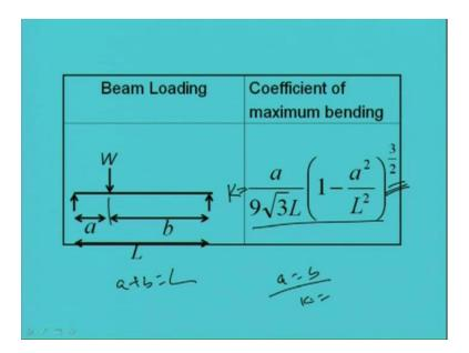
Similarly, if beam means this can be made generalized if beam is loaded at a distance from 1 side and b distance from other side where, a plus b is equal L. Then, we can find out the coefficient as a by 9 root 3L into 1 minus a square by L square to the power 3 by
