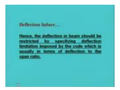
Therefore, the deflection in beam should be a restrained by specifying deflection limitation imposed by the code, which is usually in terms of deflection to the span ratio. If deflection is this, that is this then what should be the limiting value. That means, the code has guided some guidelines through which we can find out what is the limiting deflection. What is the maximum deflection can be allowed, that we can find out from the Codal provisions.
