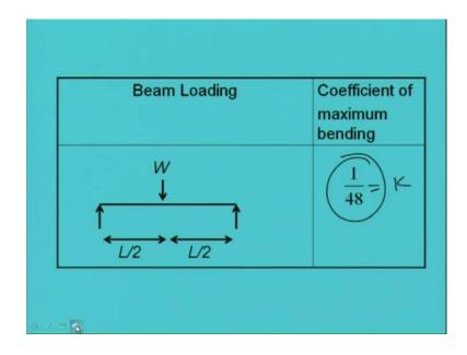
And again, if it is say beam loading is like this say L by means the load is acting at midpoint of the beam section and the beam is under simply supported condition. Then K will become 1 by 48.
