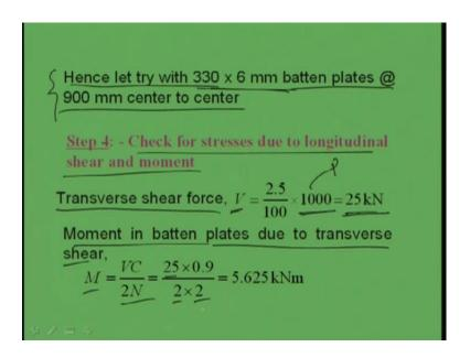
Next we can find out the stresses. So, we are going to provide this is the thing that theta t by 6 mm batten plates at 900 mm center to center. So, this is the outcome we got, right.
