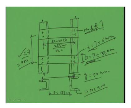
So, here D we are going to decide 330 mm. So, all the things we found thickness, depth and spacing. Now, we have to find out number and before that we have to check the stresses. So, in step 4, we will check the stresses due to longitudinal shear and moment. So, we can find out first transverse shear V is equal to 2.5 percent of the total load. This
