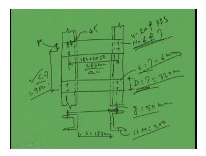
So, if we see now the details of the design, we will see that here number is four numbers of 25 rivets. 25 diameters of power driven shop rivets and four numbers means say suppose this four let us provide and this rivet distance will become 80 and this edge will become 45, right. So, in this way we are going to get all the details. So, with this I like to conclude today's lecture as well as the chapter of compression member. In the next class, we will start a new chapter.
