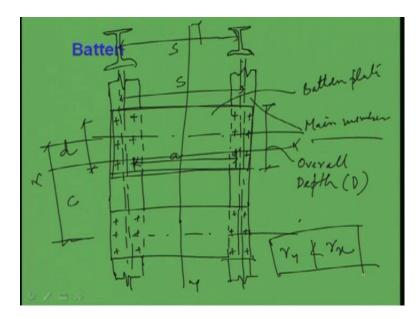
Suppose this is a section, sorry elevation of the batten plate, say here one plate is given, this is another one. This is a plate. Batten plate is here, another plate say suppose it is here. So, this is a plate, another plate is here. So, this is a compression member and this
