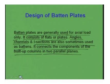
So, as I was telling that batten plates are generally used for axial load only. It consists of flat or plates. Angles, channels and I sections are also sometimes used as battens. It connects the components of the built-up columns in two parallel planes. So, how does it look let us see.
