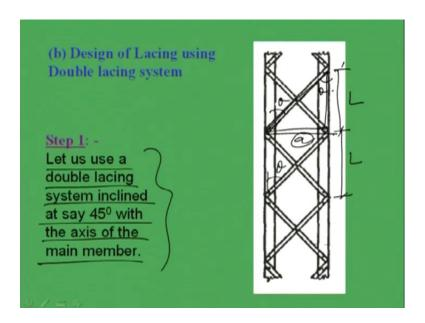
Now, the same problem we will design by the use of double lacing. That means in first half what we have seen that first we have found the built up section, appropriate build up section to carry the required amount of load that is 1000 kilo Newton. Then, we have
