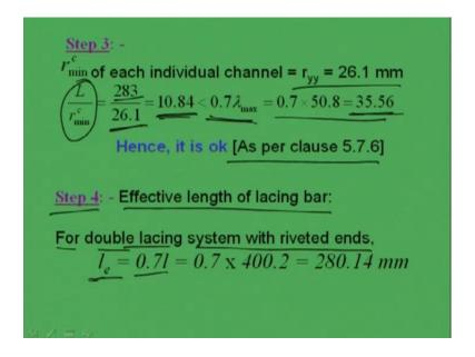
In step 3, what we will do? We will check L by rc minimum ratio which should become less than 0.7 lambda max. Here L is 283 and rc minimum is 26.1 because ryy is 26.1 from the table we got, and from this we can find out that L by rc minimum is 10.84 which is less than 35.56. So, it is completely right as per the clause 5.7.6 of IS: 800-1984.
