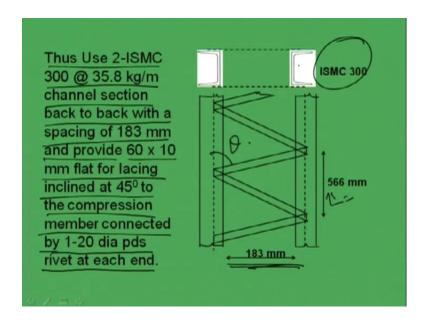
So, we can see here in short we can say that use 2 ISMC 300 at 358 kg per meter channel section back to back with a spacing of 183 millimeter and provide 60 by 10 mm flat bar for lacing inclined at 45 degree to the compression member connected by one number of 20 diameter power driven soft rivet at each end, right and if we show the drawing, we have to show that what the spacing is, what this 1 value is and of course, this theta and other things we have to show the section as such.
