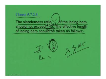
Another thing is in clause 5.7.2.3 which has been described that the slenderness ratio le by r of the lacing bars should not exceed 145, right. This is another codal provision which has been made by the code and the effective length of lacing bar should be taken as follows.
