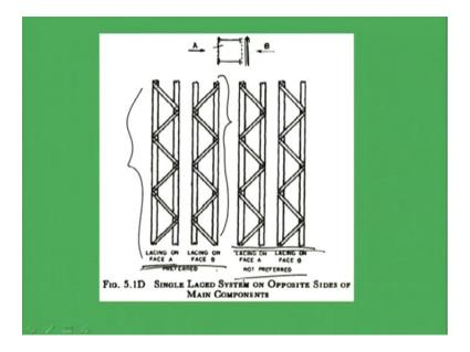
Single lacing system with AA side and this is BB side, right. Now, if lacing on face AA is like this, then lacing on face BB should be like this. Just opposite to this right, but not
