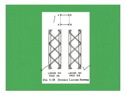
That means if we see that in case of double lacing system, this should look means face of AA, if it becomes like this and face of BB should be like this and the clause member when we are going to use it should be like this.
