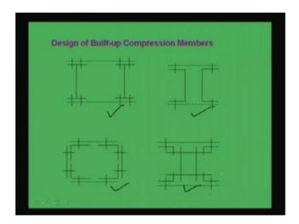
In continuation with the last lecture, we have seen that this type of members can be made with the use of individual members to find a built-up section, and the major objective of choosing the built-up section is that the radius of gyration in both the directions perpendicular to each other should be more or less equal. That means the radius of gyration in the weaker section we are going to increase, so that the strength of the member is going to increase.
