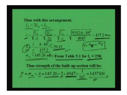
The ix value we know now radius of gyration. We know radius of gyration is ix by a or iy by a. So, ix means 2 ixx and a means area of the built-up section which is 2 into a where small a is the area of the individual section. Now, after equating we will see ixx by a. Now, if you put the value of ixx and the area of the individual section, we will get r as 137.2 millimeter, right and this is also directly we can find out from the SP6, right. So, lambda will become l by r.
