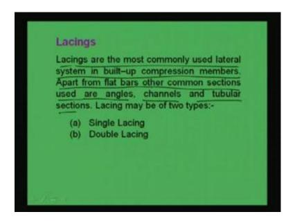
So, we can see that lacings are most commonly used lateral system in built-up compression members. Apart from flat bars, other common sections used are angles channels and tubular sections. So, for lacing, generally we use flat bars. Other than that we use also channels, tubular section or angle sections. Now, lacing can be divided into two types. One is called single lacing, another is called double lacing.
