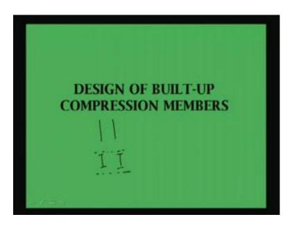
Suppose we have say two I sections. Then, we will see that this is a battening or lacing. Now, if we see in the elevation, we will see that this acting something like this. That means we will be having some sort of lacing like this. Then, this is called lacing system ((lattice)) members we have to provide. We will come to details later.
