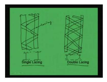
What is single lacing? Let us see. Single lacing if you see say two I section is there, right. Suppose these are the two I sections. Now, the lacing is provided here. So, if the elevation, this is one I section, this is another I section, right. So, what we will do? So, this is how lacings are placed. This is called single lacing. This is the lacing and in case of double lacing, what will happen.
