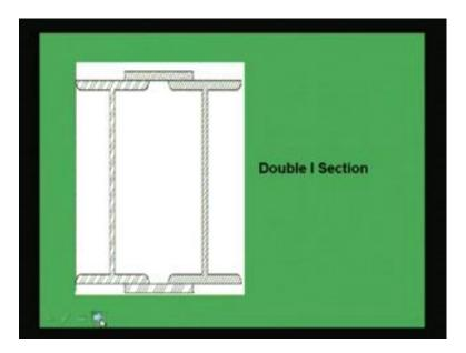
Another section which is commonly used as double I section as we have shown earlier. Double I section connecting through lacing or battening or some plate, right.
