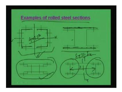
Now, some examples of rolled steel section with built up section. So, as we say suppose this is a angle section, this is another angle section, this is another angle section and this is another angle section. So, if we arrange four angle sections with box like things, then here Ixx and Iyy both will become very high. Ixx means in this direction X and Iyy means this direction. So, the radius of gyration will become more in this case. That is why this type of section is preferable.
