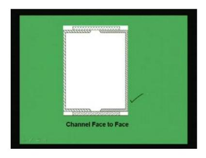
Another common section is the channel when comes face to face. We will see what is the advantage or disadvantages or which type of section we should go for a particular case of design. We will see later when we will go for designing.
