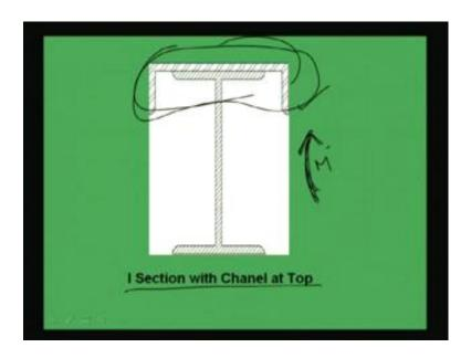
Another section available is that I sections with channel at top. If the stress is coming more here means in this side if moment is like this, moment is acting in this direction, then the compressive stress will be acting more here, coming more. So, in that case we may need some extra material which can be provided in terms of channel also. This is one section which is also commonly used in the industry.
