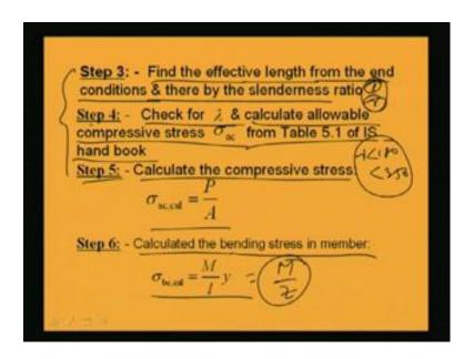
That means find the effective length from the end condition, and there will be a slenderness ratio with the new section. Then, we will go through these steps. So, unless the condition has been satisfied, we will go on increasing the size of the section and we will therefore be able to get a suitable section. So, this is the design procedure. Now, if we go through one example, we will be able to understand how to design a beam column like members.
