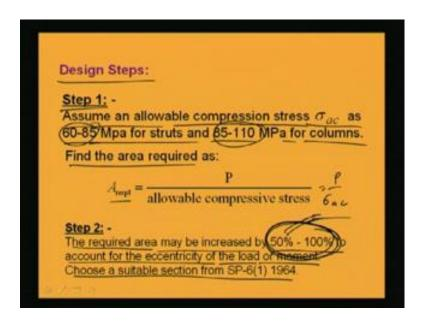
Now, I will discuss the design steps which have to follow for design of a beam column type member. So, in first steps what we will do? We assume an allowable compression stress sigma ac as 60 to 85 MPa for struts and 85 to 110 MPa for columns. As we have discussed in last class also that we will consider 60 to 85 MPa for struts and 85 to 110 MPa for the column members. This is the starting point.
