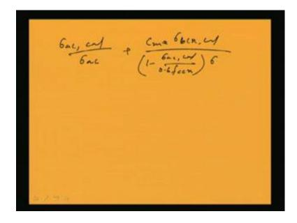
So, we have to use the earlier formula that is sigma ac calculated by sigma ac plus Cm x sigma bcx calculated by 1 minus sigma ac calculated by 0.6 fccx into sigma which is less than 1.0.
