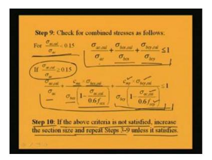
Then, we will see that whether it is less than 0.15 or greater than 0.15. If it is less than 0.15, the expression has to be satisfied. What is this expression? That is sigma ac calculated by sigma bcx plus sigma bcx calculated by sigma bcx plus sigma bcy calculated by sigma bcy should be less than or equal to 1. If the ratio of sigma ac calculated by
