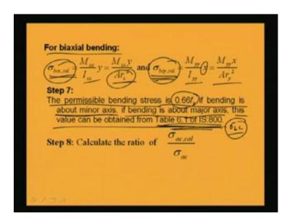
So, after getting this sigma bc, what we are getting? Sigma bc in x and y direction in minor about minor axis, this will be 0.66fy and about major axis, this will be finding from table 6.1. Now, we will find out ratio of sigma ac calculated by sigma ac.
