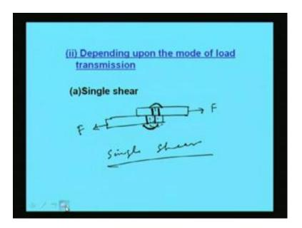
So, how does look the single shear joint? That means, 1 plate is like this and another plate will be like this. So, single shear means it is like this it should be, but if failure occurs then what will happen, so this will come here right. So, in case of single shear this failure will be in this way right F this is called single shear right. So, the failure of the single shear will be like this.
