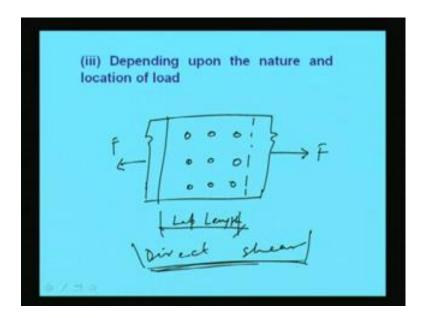
So, if we see the shear connection how it will look that means if 2 plates are over lapped and comes under tension say F and this F with a lap length of l say lap length and with having say. Then this is this will come under direct shear, so this will be calculated the strength of the joint will be calculated under this condition that it is withstanding the direct shear. So, accordingly how much shear is going to be developed due force F and how much how many, number of rivets will be required.
