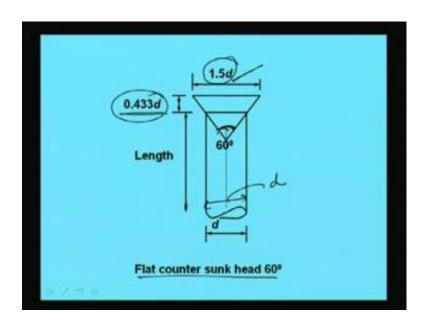
Another is flat countersunk head 60 degree flat countersunk head 60 degree; that means, here the angle will be 60 degree and the width of this head will become 1.5 d and the height of this head will become 0.433 d right. So, if the d is the nominal diameter of the sunk the, if this is d then the width of the head will become 1.5 d. And height of the head will become 0.433 d and the angle between these 2 will become 60 degree.
