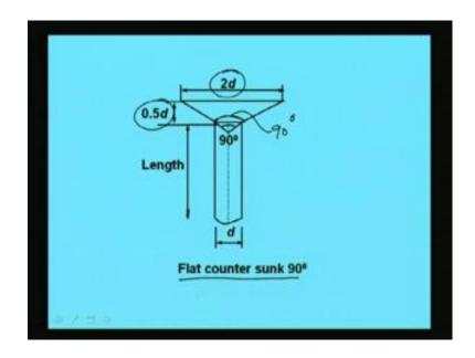
Another type of rivet is called flat countersunk 90 degrees in case of this the dimensions are given like this that the height of the head will become 0.5 D. And the width will become 2 D and the angle between these 2 will become 90 degree, so in this way it has been designated.
