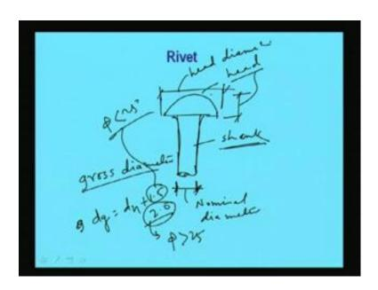
If we see it has a head and another part is called shank, so this is called shank and this diameter is called nominal diameter. And this head and this is. In fact, this is called head diameter and this height this height is called basically. So, a rivet consist of shank and head shank the length of the shank depend means will decided on the thickness of the plate how much it is required accordingly shank would be decided. Now, nominal is
