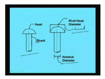
So, the rivets look like this one is nominal diameter another is rivet diameter, and this is called a head I mean this is rivet head diameter and this portion is called shank.
