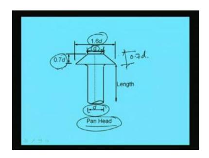
Another type of rivet is called pan head, in this pan head the head is look like this. Here if the diameter is D then the height will be 0.7 d like the previous one like the snap head the diameter 0.7 d here the height also is 0.7 d. And the width will be 1.6 d here maximum width will be 1.6 d and here the width will be D this is D right. So, the specialty of pan head is that the head will be 0.7 d and the width maximum width will become 1.6 d where the width at the top will become D.
