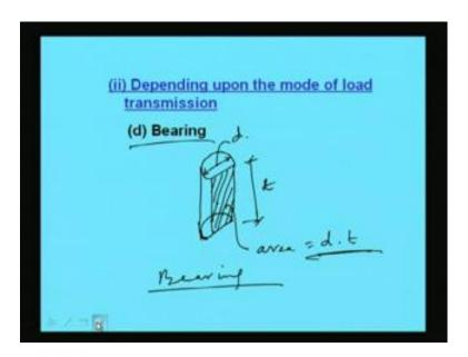
Another type of failure is called bearing in case of bearing what it will look this will look like this now, this will look like this right. So, this is the length, so failure will be due to bearing, so this is the diameter d and this is the say thickness of the plate if it thickness t. Then the total area this area will become d into t D in to t dt, so this will be the area, so this failure is called failure due to bearing.
