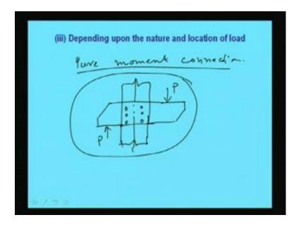
Another case will be happen when pure moment will come into picture and the connection will be called as pure moment connection. That means when it will come if the members are like this say this is a column which is taking the load like this right now, this p and this p. So, rivet is given here now, this type of connection is called pure
