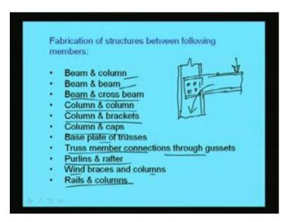
Then say beam and beam beam and cross beam then column and column column brackets columns and caps like this base plate truss members. And then purlins and rafter wind bases and columns rails and columns I am just showing 1 picture say suppose 1 column is there and another beam is here. So, how to connect it? So, this is a column and this is a say beam now, connection has to be made. So, what we use to do? That connections can be made either temporary or in permanent in nature.
