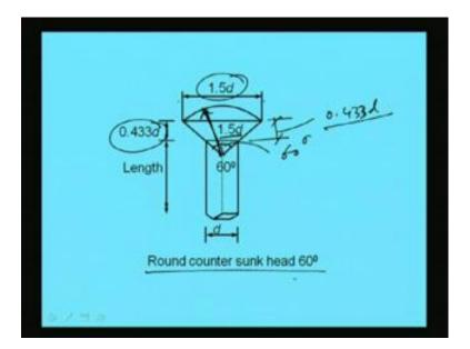
Another type of rivet is called round countersunk head 60 degree round countersunk head 60 degree here the angle between these 2 will become 60 degree. And the this
