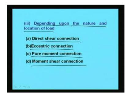
Another is depending upon the nature and location of load depending upon the nature and location of load. So, this will be 1 will be direct shear connection we can make another is eccentric connection pure moment connection and moment shear connections.
