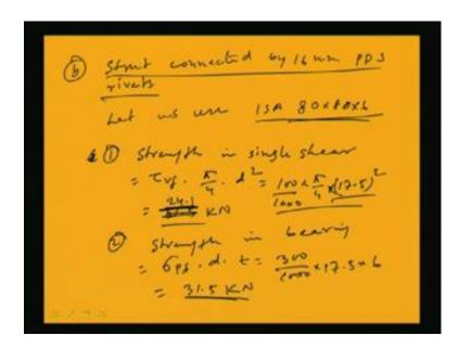
Now, let us see the second case if the strut connected by 16 mm power driven soft rivets. Now, with these strut connections, let us see how the design is going to vary. So, now let us first use say previous section 80 by 80 by 6 which was unsafe. For earlier case, let us use ISA 80 by 80 by 6 sections which was unsafe in the previous connection. Now, we will see whether this is safe or not. If it is not safe, then we can go for the next section.
