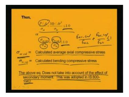
So, we can write the earlier equation as P by A by sigma ac plus My by Ar square by sigma bc which should be less than or equal to 1. That means if we divide this A with this equation, then we will get this one. If we divide the A with both the sides, then we will get P by A by sigma ac and My by Ar square by sigma bc which will be less than or equal to 1, or we can write P by A is nothing, but the sigma ac calculated. So, sigma ac calculated by sigma ac plus.
