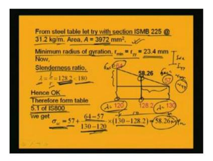
So, from steel table let us try with IS MB 225 of 31.2 kg per meter. So, for that particular section area is 3972 millimeter square. We need area 3750 millimeter square and we have area 3972 millimeter square. So, the moment we find out an appropriate section for the trial case, so what we will find. We will find out what the minimum radius of
