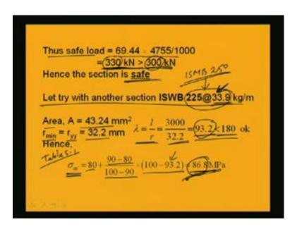
Thus, the safe load can be found out now that the area into this. So, if we calculate this is you are going to get as 330 kilo Newton, right. So, the area we will be getting as 330 kilo Newton which is greater than the given load which is 300 kilo Newton. So, we can say that the section is safe. So, what we have seen that if we choose ISMB 250 section, then the section can carry the given load which is 300 kilo Newton. In fact, the load carrying capacity of that section is 330 kilo Newton.
