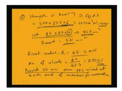
Similarly, strength in bearing will be sigma pf into d into t. So, for power driven soft rivets sigma pf value will be 300. Here d is 23.5 and t is the thickness. So, for thickness, the plate thickness we have to make, sorry the member thickness. So, let us assume member. Before that we have to assume a member say ISA 80 into 80 into 6. Let us assume this because to take care of the required area was given as 571 millimeter and this area is given as 929 millimeter.
