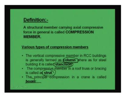
Again if same type of member is used in the steel building, then this is called as stanchion. The compression member in roof, truss or bracing is called strut and the principal compression member in a crane is called boom. That means, the same compression member is termed different way. One is column or stanchion or strut or boom. Like this we used to generally term them.
