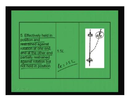
This is another condition where it has been told that effectively held in position and restrained against rotation at one end. That means this one and at the other end, partially restrained against rotation, but not held in position. In this case, the effective length can be calculated from this formula that is le is equal to 1.5 L.
