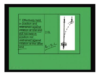
Another option which is given here that effectively held in position and restrained against rotation at one end means, restrained against rotation and position, but not held in position nor restrained against rotation at the other end. This is free. So, at the other end, it is not restrained against rotation and nor the position. So, in this case, the length will be 2 L, right. So, like this the effective length for different cases can be calculated, right.
