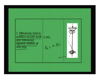
Another case may appear which is like this. That is one hinge in one end and another end is fixed which can be defined as effectively held in position at both ends and restrained against rotation at one end. That means, effectively held at position at both ends and restrained against rotation at one ends. Here against rotation, it is restrained, but here it is not. That means, in one end it is hinged, another end it is fixed. So, in this case the effective length will be 0.8 L, right.
