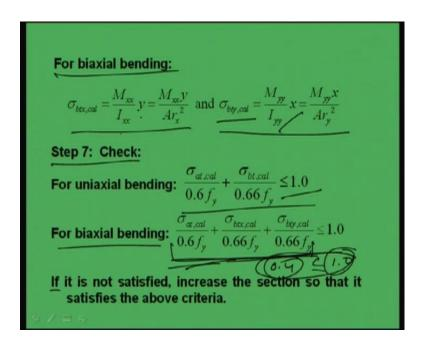
For biaxial bending, we have to calculate the two type of stresses sigma bt x calculated and sigma bt y calculated, right. Sigma bt x will be Mxx by Ixx into y and sigma bt y calculated will be Myy by Iyy into x. So, now we have to check the following condition. This is one condition for uniaxial moment that is sigma at calculated by 0.6fy plus sigma bt calculated by 0.66fy which should be less than or equal to 1 which we have discussed earlier.
