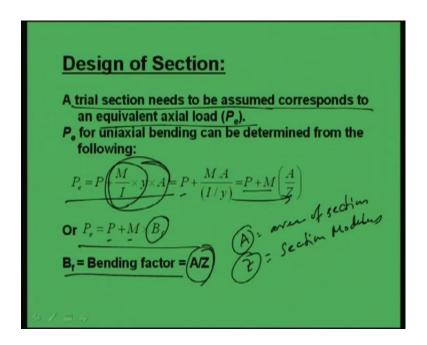
Now, let us go to the design. So, how to design the section? Now, in this case first we have to go for a trial section because we do not know which section we have to go. We have only the load and moment. So, through iteration we have to find out a suitable section. So, one way we can make that equivalent axial load, we can find out M. A trial section needs to be assumed correspondence to equivalent axial load, so that equivalent axial load can be written from this.
