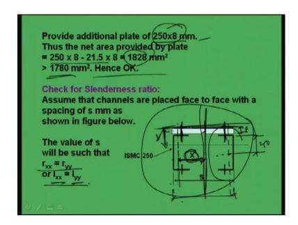
So, we have to provide some plate. So, we are providing plate here say of 2550 by 8 millimeter plate. Now, if we provide this plate, then net area can be found because rivet joint has to be made. If we make rivet here, then we will see that 215 to 8 minus 21.5 into 8, this will be becoming net area which is greater than the required one. So, providing this much plate is sufficient to take care the load.
