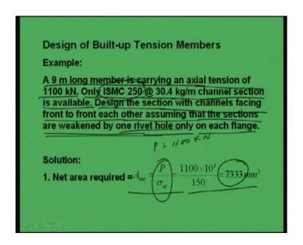
Now, question is that a 9 meter long member is carrying an axial tension of 1100 kilo Newton. Only ISMC 250 at 30.4 kg per meter channel section is available. Design the section with channel facing front to front each other assuming that the sections are we can by 1 rivet whole only on each flange. The assumption is that only one rivet has been
