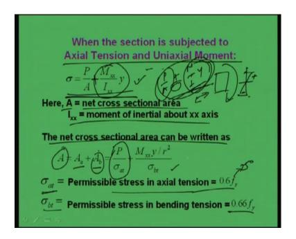
Now, how to analyze and design when the member is subjected to axial tension and say uniaxial moment? Now, there are two scope means one is axial tension and moment in one direction. Another is moment in two directions along with axial tension. That means axial tension along with biaxial moment. So, both the cases we will see.
