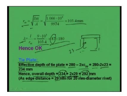
So, now we will find out the rxx which is nothing, but Ixx by A or Iyy by A. So, this is becoming Ixx by A is becoming 103.4 radius of gyration, and the slenderness ratio is nothing, but I by rxx. So, length is given 9 meter and radius of gyration is 103.4. So, this is becoming 87 which is less than 180 as per the codal provision if it is less than 180. So, from the slenderness ratio point of view also, the assumed section is to take care of that much of load, right. So, this is fine.
