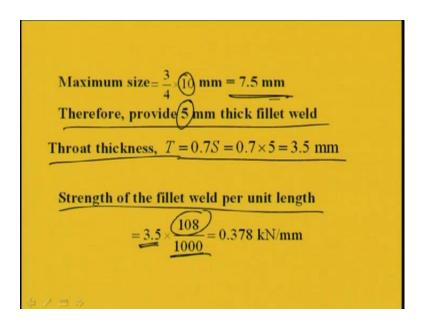
And maximum size for this case can be used three-fourth by t; t is the thickness of the angle which is 10, so 7.5. So, in between 3 to 7.5 mm, we have to find a fillet weld size. So, what we will do? Now fillet weld size we are providing in between as 5 mm. So, if size of fillet weld is 5 mm, then throat thickness can be found out from 0.707 or 0.7 S; that means 3.5 mm, right.
