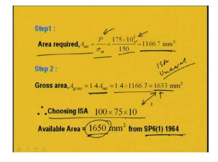
Now as we have discussed, what is the steps one? In step one, first we will find out the required net area. Net area required will be P by sigma a t, where P is the force applied and sigma a t is the allowable tensile stress on the member. So, load is 175 kiloNewton; we are making it Newton, and this is 150 Newton per millimeter square. So, net area required is 1166.7 millimeter square.
