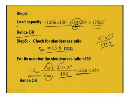
So, 1266 millimeter square and we need require as 1166.7 millimeter square. Net area is required 1166.7 millimeter square. And available net area we are going to get 1266 which is greater than the net area required. So, we can go with this section, right. Load
