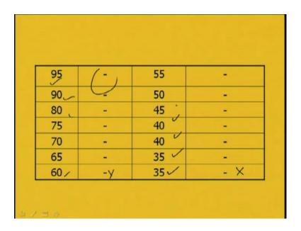
So, similarly again we see for different angles; means below 100 mm leg size, we are not going to provide double row. In that case, we are going to provide only single row. So, the gauge line will be here, and there will be no double rivet; that is why nothing has been provided.
