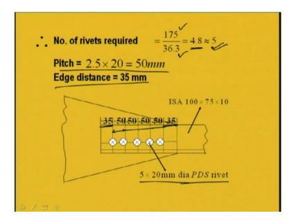
Next what we will do? Now number of rivet required; so number of rivets will be load by rivet value; load is given as 175kilo Newton, and rivet value is 36.3 kiloNewton. So, number of rivet required will be 4.8; that means 5. So, five number of rivets can be used for this, right. Now pitch, pitch from the codal provision we know minimum pitch will be 2.5 into D that is around 50 mm. So, we can make 50 mm. And edge distance, say let us consider 35 mm, right.
