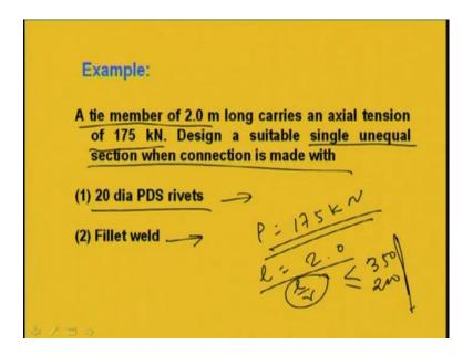
First, I will go through one unequal single angle section, say a tie member of 2 meter long carries an axial tension of 175 kiloNewton, right. So, axial tension is 175 kiloNewton. Now design a suitable single unequal section when connection is made with 20 mm diameter of power driven soft rivets and fillet weld. So, we will design through fillet weld, we will design through riveting 20 mm diameter of power driven soft rivet.
