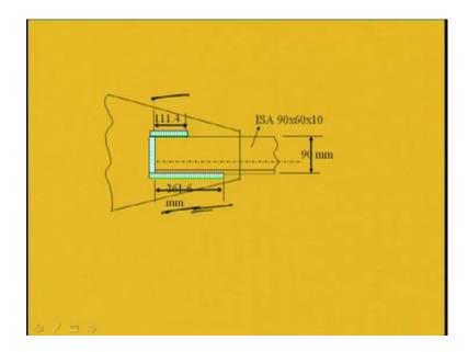
So, the design will be like this that this is 261.6 millimeter; this is 111.4 millimeter, and this is 90, right. So, the welding if we distribute in this way, then the CG of the weld and cg of the section will coincide each other. So, there will be no scope of eccentricity. So, in this way we can make design.
