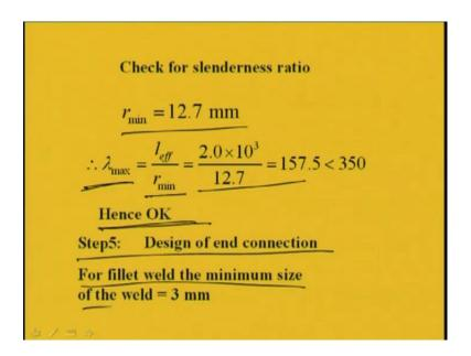
Now again the slenderness ratio has to be checked. So, for that section from the SP 6, we will get the minimum r is 12.7 millimeter; for a particular section, the radius of gyration minimum maximum along with all the member properties has been given in the code SP 6. So, lambda max will be I effective by r minimum. So, this is becoming 157.5 which is less than 350; that means it is safe.
