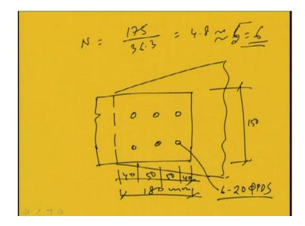
Number of rivets will be, say 175 kiloNewton load has to be provided; 36.3 is the rivet value is 4.8, say let us provide. Say, this will be basically 5. So, as two rivet in each row has to be provided. So, let us provide six rivets, right. So, provide six rivets and with a pitch distance of 50 and edge distance of 40 mm, right. So, number of rivets is becoming. So, what we are going to get that if we now draw. So, this will be now we can make one, sorry.
