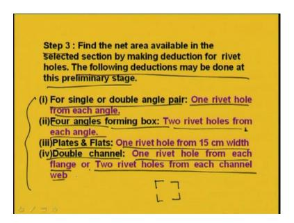
Next, the step three is that find the net area available in the selected section by making deduction for rivet holes; that means we know the rivets are there. So, deduction due to rivet hole has to be made. So, the following deductions may be done at this preliminary stage. So, some guidelines we have. So, these are the guidelines through which we can deduct at the preliminary stage.
