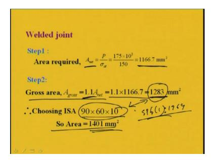
Now we will go for welded joint. So, same problem we will go through welding joint. So, in case of welded joint again we will see how to find out. First, what we will do? That net area we have to find out P by sigma a t which is 1166.7 millimeter square. Now gross area for welding joint because gross area will not be much, because in case of welding joint, there is no scope of deduction of hole. So, net area and gross area will be almost nearby.
