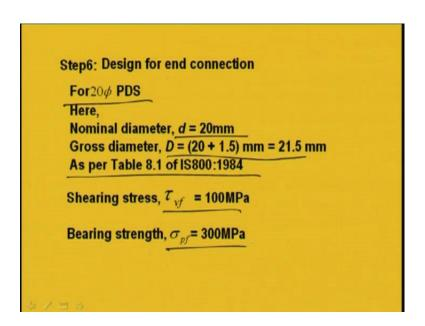
Now what we will do? Next step is design for end connection. So, we are using 20 mm diameter of power driven soft rivet. So, what we will do? So, nominal diameter will be 20 and gross diameter will be 20 plus 1.5 that is 21.5 And as per table 8.1 for power driven soft rivet, tau v f is this and bearing strength sigma p f will be 300 Mpa and tau v f
