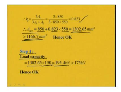
K 1 is equal to as we know 3 A 1 by 3 A 1 plus A 2. So, providing the value of A 1 and A 2, we can find out the magnitude of K 1 as 0.823. Now area net, net area will be becoming A 1 plus K 1 into A 2. So, A 1 is 850, K 1 is 0.823, A 2 is 550. So, after calculating this we are going to get 1302.65 which is greater than the required area; required area was 1166.7 millimeter square. So, it is okay.
