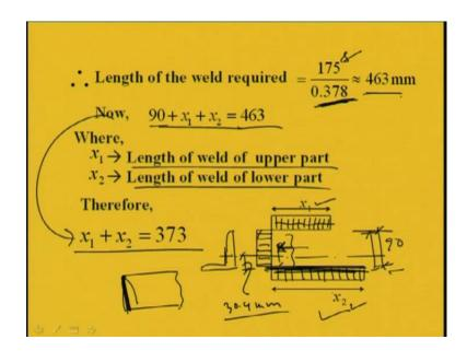
Length of the weld required will be this one because this is the load which has to carry by the weld and 0.378 kiloNewton per millimeter length is the strength of the weld. So, if we divide it, we are going to get 463 millimeter. So, length of weld is required 463 millimeter, right. So, 463 millimeter length has to be provided. Now how do we provide? Now we see when the member is here. So, what we will do? First, we can provide that this is the length of the connected leg.
