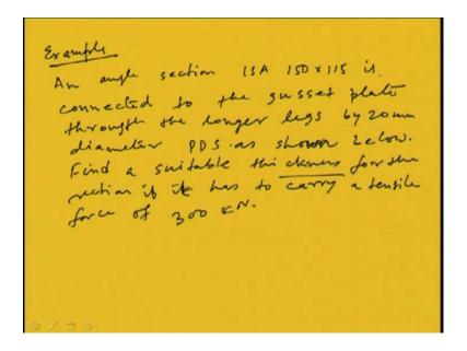
So, this is the question. Basically, this is one sort of design also you can say that an angle section of ISA 150 by 115 is connected to the gusset plate through the longer legs by 20
