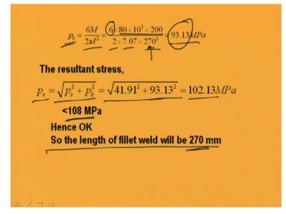
Again p b, p b will be 6 M by 2 t d square; so 6 M by 2 t d square. So, moment is p into e 80 into 10 cube into 200. So, 6 into this by 2 t d square; so this is becoming 93.13. Remember, this p b we have considered earlier as 108, then we are getting the d as 251. Now as we have increased the length up to 270 that is why the stress due to bending is coming less than 108 which is 93.13.
