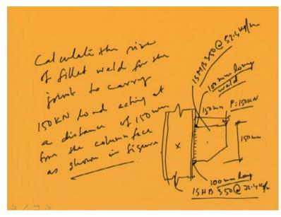
One column has to carry some load of, say 150 kiloNewton, say P is equal to 150 kiloNewton. And this eccentricity is, say 150 mm. Now this has to make the welded joint and this is the column flange we are making. Now this has to make the welded joint here, right, throughout this depth. Now this depth is 150 mm and here 100 mm long weld is also provided horizontally. Here also 100 mm long weld has been made.
