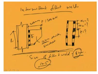
That is about the intermittent fillet weld. What is that? It is the analogous to the rivet joint; means basically if we see in a line that after some gap some welding has been done with some gap. So, this is called intermittent fillet weld. Now with the use of intermittent fillet weld, we will see one example. Say, if we consider one example, say this is one intermittent fillet weld. This is seen in the plan; that means we are making welding with a particular pitch distance.
