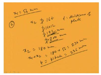
So, I can write x 1 as, finally, x 1 will be 56 mm. Because when I am talking that x 1 as 56 mm; that means the actual length is 56 minus 2 s; that means 40 mm, right. Next we will do x 2; that means clear spacing between that two adjacent intermittent.
