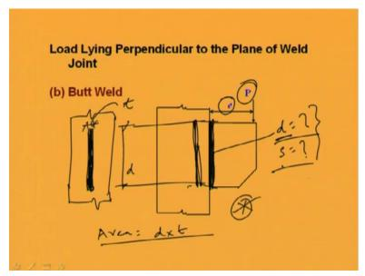
That means this depth and this depth and size. So, basic thing is depth we have to find out. So, how do find out this depth? How much depth or length we have to make weld to carry a particular load within particular eccentricity. So, this d has to be found out as well as if d is given, again the size of the weld has to be found out. So, both the things if it is unknown, we have to assume one thing and then other things we can find out.
