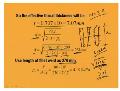
So, using same size of the fillet weld as in case of butt weld, let us see how much depth we are going to get. So, the effective throat thickness will be 0.707 into s size. So, this is becoming 7.07 millimeter effective throat thickness. Now d; d will become from the equation if we see if from plan we see, this is the fillet weld is generally made in this way. In two sides, weld has been done. So, the area and the other things will be different from the butt weld.
