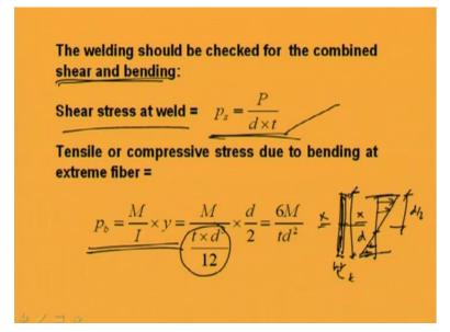
Now shear stress will become P by d into t because area is d into t. So, now the welding should be checked for combined shear and bending as we know because of the eccentricity of the joint, the bending as well as the direct shear will come into picture.
