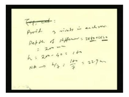
So, with this I can find out tall v f cal. Sorry, provide three rivets in each row. So, what will happen? So, depth of stiffener can be found out. That will be 2 into 60 plus 2 into 40. Edge distance we are considering 40 and pitch is considered 60. So, with this we are getting 200 mm. So, h will become 200 minus 40; that means 160, right. So, neutral axis will be lying at h by 7; that means 160 by 7; that means at 22.9 mm from the bottom, right. So, how does it look like?
