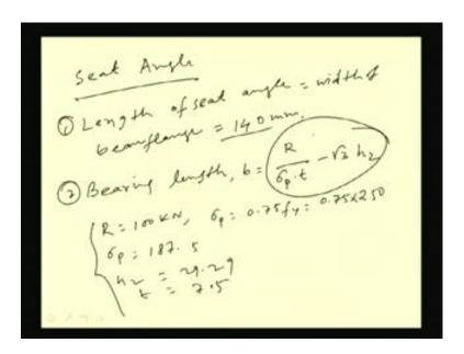
So, for seat angle length has to find out. So, length of seat angle this will be basically will be equal to the width of beam flange. So, that is given as 140. So, length of seat angle it has assumed as 140 mm. Now we have to calculate the bearing length next step. So, first step is this; say next step is bearing length which is called b; that is it can be found out from this formula R by sigma p into t minus root 3 into h 2.
