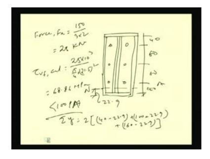
So, if we see we will see. So, we are using three rivets, right, and these are 40, 60, 60 and 40, and neutral axis is lying here, neutral axis which is 22.9, right. So, now force in each rivet due to direct force, force in each rivet f a will be total load by total number 150 by 3 into 2. That will become 25 KiloNewton. So, now tau v f cal can be found out 25 KiloNewton by area of the rivet pi by 4 into 21.5 square.
