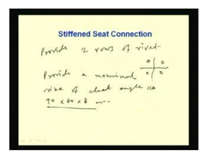
So, let us make that provide two rows of rivet. That means two rows means we are providing four, right; four rivets we are providing. So, total number of rivets is becoming four. This is all about the seat angle. Now cleat angle we have to make. So, provide a nominal size of cleat angle, say ISA 90 by 60 by 8, okay. So, cleat angle we are providing this 90 by 60 by 8. And we are providing some this rivet to join the cleat angle between column and the beam.
