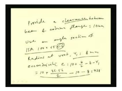
Next what we will do? We will provide some clearance; that means gap. We have to assume some clearance; say provide a clearance between beam and, say column flange, okay. So, 10 millimeter gap we are providing. Provided clearance between beam end column of a clearance, say this we are providing as 10 mm, okay. And let us use an angle section because we have to assume some angle and then we have to check angle section of, say ISA 100 by 65 by 10, okay.
