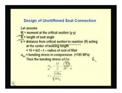
If the moment at the critical section is assumed as M and the length of seat angle is denoted as B. Then we can find out sigma b c as M by Z, where M is nothing but R into e; that means R is the reaction that is given, because of the load coming from the system coming through the beam or girder whatever you say. So, R e will be; that means e is the eccentricity that is distance from critical section to reaction acting at the center of bearing length.
