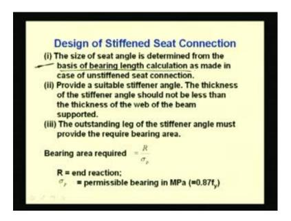
Now we will discuss about the design of stiffened connection. So, for design of stiffened connection means stiffened seat connection, almost similar way we will find out the design process except the design of stiffener. So, first step is that the size of seat angle which is determined from the basis of bearing length, okay, as made in case of unstiffened seat angle. So, the size of seat angle we will make as similar to the unstiffened seat connection; this is first.
