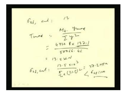
So, I can find out now sigma t f cal which is sorry. So, M t I am going to find out this. So, now T max will become M t into y max by summation y square, and y max will be the outermost rivet. So, that will be 4930.8 into 137.1 by 50066.46, because y max is this outer most. So, from this I am getting 13.5 KiloNewton. Now sigma t f cal can be found out now 13.5 by area t by a 5 by 4 into 21.5 square. So, this is coming 37.2 MPa which is less than sigma t f which is 100. So, it is okay.
