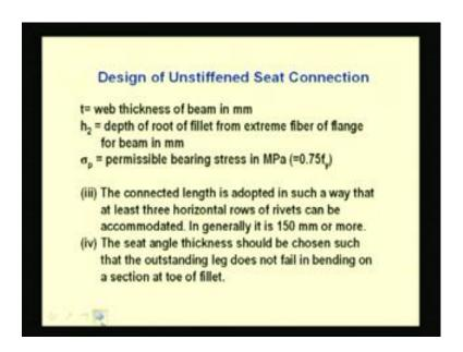
Now t is the web thickness of beam in millimeter. Here we are using t sigma p h 2 along with R. So, t is the thickness of the web of beam in millimeter. H 2 is the depth of root of fillet from extreme fiber of flange for beam in millimeter. This has been given in the code; in SP 6 all the details has been given. That means for a particular angle whichever we are going to consider seat angle whatever we are going to consider, for that particular angle we have all the details.
