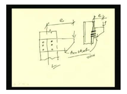
So, in case of bracketed connection it looks like this. We have seen that the load is coming from a girder or from somewhere else, and it is transferring to the column through this bracket; this is called bracket. And whether it depends on that bracket depends on whether load is lying on the plane of rivet joint or the load is lying perpendicular to the joint. If it is perpendicular to the joint, then we know how to means make it.
