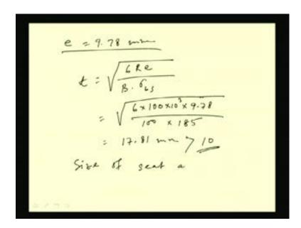
So, the eccentricity we are getting 9.78 millimeter, right. Now we will find out the thickness required to withstand that much load. So, thickness can be calculated from that formula that is 6 R e by b into sigma b s and the allowable stress sigma b s will be 185. So, 6 into r means 100 KiloNewton; that means 100 into 10 cube. E is 9.78 millimeter which has been calculated. And b is the width which is 100. And sigma b s is the permissible stress in bending that is 185, right.
