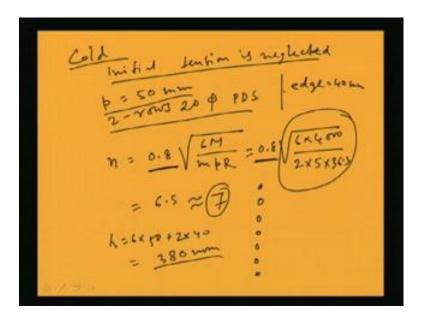
Now another example we will do that is cold rivet; means same example with the assumptions of rivet as cold; that means initial tension is neglected. So, if initial tension is neglected, how to calculate? So, what we will do? So, similarly we are considering the pitch distance as 5 centimeter means 50 millimeter center to center and two rows of 25 power driven soft rivets. These are the assumptions means we have considered.
