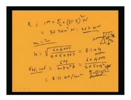
Second thing is rivet value. Rivet value will be tau v f; that means 100 into pi by 4 into d square. 200 mm diameter of rivet has been used. So, its gross diameter will be 21.5. So, from this I can find out Newton. This will become 36.3 into ten cube Newton; that means 36.3 kiloNewton. So, rivet value we have. Now here m will become two because two line of rivet has been provided. So, all the values now we have. So, I can find out the value of n. Six m.
