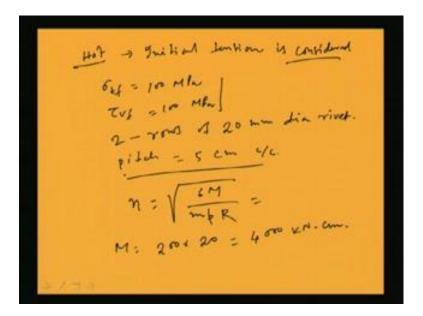
So, first thing is that we are considering power driven rivet. That means initial tension is considered, because of hot driven rivet, initial tension will be there. So, we are considering initial tensile is there, okay. So, for power driven shaft, we know from the codal provision that sigma t f will become 100 Mpa and tau v f with 100 Mpa; these are the things which we know from the codal provision.
