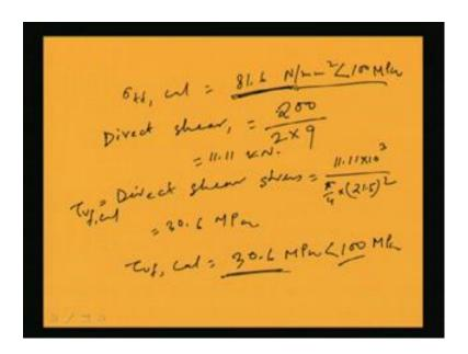
Now that means sigma t f calculated will be 81.6 Newton pe9r millimeter square. If I change the unit it will be 81.6 Newton per millimeter square. Now, again direct shear we have to find out. Direct shear in each rivet can be found out as the force was 200 kiloNewton and number of rivets is 2 into 9. So, this is coming 11.11 kiloNewton. So, direct shear we can find out from here; this is kilo Newton.
