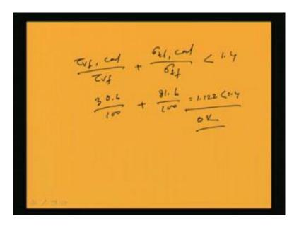
Now, jointly we can see that this equation has to satisfy tau v f calculated by tau v f plus sigma t f calculated by sigma t f; this has to become less than 1.4. So, if we put the values; this is tau v f is 30.6 by 100 plus 81.6 by 100. This is coming 1.122 which is less than 1.4; that means it is completely okay. So, in this way I can make it. So, now the thing is that we have to design; means design means we have to make all other specifications; that means we have to draw the connections.
