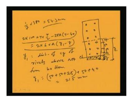
Suppose, say this is a rivet joint we have. So, we have total number of rivets we know that is 3 3 6 7, three, four, five, six, seven. And the approximate neutral axis depth we have calculated that is 1 by 7 into 380; that means 54.3 mm from bottom. Now to calculate the actual neutral axis depth which is y distance above the means from the bottom. If neutral axis depth is y, then we can write 2 into 100 into y into y by 2.
