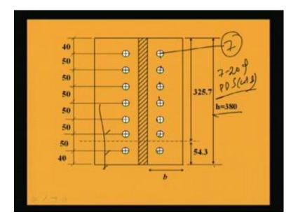
So, now we can make the diagram that we need seven number of rivets. So, one, two, three, four, five, six, seven; seven number of rivets has been used and seven number of 25 power driven shop rivets cold has been used, where the total depth will become 380 mm. And the distance between rivets and edge distance has been given in this that is 50mm, 40 mm and so on. So, in this way we can make. So, this is all about the design of riveted joint. Riveted joint can be designed in this way.
