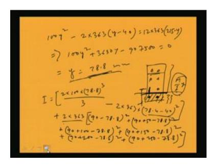
So, the equation of y to find out y, final equation will become 100 y square minus 2into area means 363; that is pi by 4 into d square into y minus 40 is equal to 12 into 363 into y 1 means 215 minus 1, okay. So, from here I can find out the equation as 100 y square plus 3630 y minus 907500 is equal to 0. So, from this I can find out y is equal to 78.8 mm.
