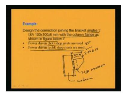
Now let us see this example that designs a connection joining the bracket angles 2 ISA 100 by 100 by 8 mm with a column flange as shown in the figure below. If power driven shop rivets are used and if power driven cold shop rivets are used. That means we will solve this problem using first power driven hot rivets and then power driven cold rivets.
