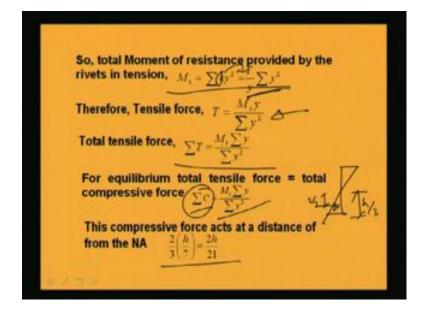
So, total moments similarly I can find out that summation of k y square and if putting the value of k as T by y, we can write T by y into summation y square. And similarly, the tensile force can be found out from this formula that M t y by y square. Then total tensile force also can be found out by summing all the moments. So, total summation will be M t into summation y by summation y square.
