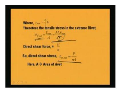
So, in this was I can find out that sigma t f cal. So, in this way I can find out sigma t f cal and tau v f cal from which I can make it. So, all this will be clear if we go through one example.
