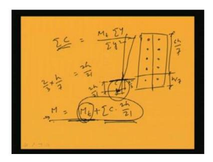
So, with this equilibrium equation we can write that total compressive force will become nothing but same that is M t into summation y by summation y square. So, in this way I can find out the total compressive force. Now if I see the diagram that if rivet groups are like this and suppose these are the plate. Now this is the neutral axis where it has passed. So, this is basically h by 7, and this is basically 6 h by 7; this is the assumptions.
