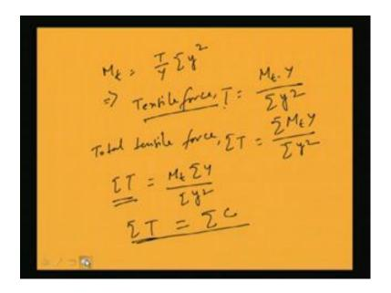
That means M t I can write in place of k, I can write again T by y. So, M t is equal to T by y into summation y square. So, means theoretically I can write the tensile force in this way tensile force T will become M t into y by summation y square. So, tensile force can be calculated from this. Now total tensile force I can write that this is a tensile force for a particular rivet. So, total tensile force this also can be calculated.
