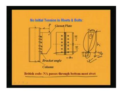
Now before going to start the analysis, we will see that as I have told earlier also that the neutral axis we are assuming that it will be if the total depth of the joint is h, the section is h, then h by 7. The neutral axis is assumed to be at h by 7. This assumption has been made by US code and as well as our Indian code also is also following this assumption that at h by 7, this neutral axis will move.
