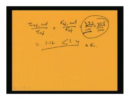
So, in this way I can find out the total value this tau v f calculated by tau v f plus sigma t f calculated by sigma t f is equal to 39.3 by 100 plus 72.5 by 100. Now you see this means tau v f has to be less than 100 and sigma t f also has to be less than 100 first thing. Second thing is this total summation should be less than 1.4. This is coming around 1.12 which is less than 1.4. So, I can make it as okay. So, in this way I can check.
