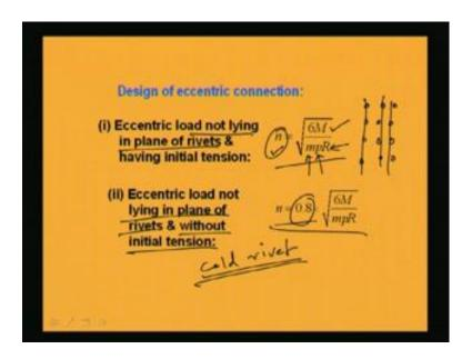
Now for design of eccentric connection when the loads are not lying in the plane of rivets, we have seen earlier also that we can assume this formula that n is equal to root
