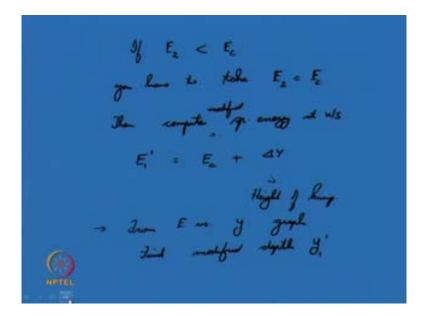
So, if you are computed E 2, comes less than E c, you have to take E 2 is equal to same as the critical energy flow, or the energy at the specific energy at the critical flow. Then compute specific energy at upstream, this is the modified specific energy at the upstream section; E 1 dash, this is nothing but E c plus del y, del y is the height of hump. So, once you compute E 1 dash from E verses y graph, find modified depth y 1 dash at section 1 1.
