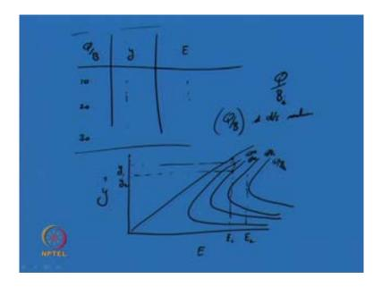
If I try to interpret say, for different Q by B, for different depth of flow, and E if I try to compute it in a table, so you can start with Q by B is equal to 10 20 30 from then from different depths E, like this if you try to compute them, you will see there you are going
