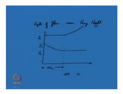
You can easily see that, if I plot depth of flow verses hump height, as we have assumed that initially at the upstream section, the flow is sub critical. So, you can just see for the
