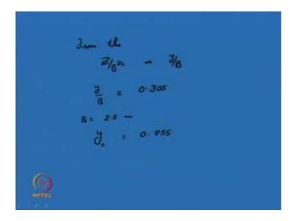
So, from the z by B to the power of 5 by 2 verses y by B graph, you got y by B approximately around 0.305 or something, B is equal to 2.5 meter. Therefore, your critical, your critical depth of flow is around 0.755 meter something like this. Like this
