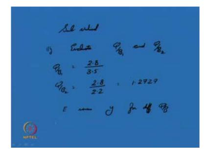
Similarly, evaluate Q by B 1 and Q by B 2, you know Q by B 1 is equal to 2.8 by 1.1, Q by B 2. Well I beg pardon, Q by B 1 is 2.8 by 3.5, and here this 2.8 by 2.2. So, you have the respective curves of Q by B, is a you have the respective curves of E verses y for different Q by B, you obtain those thing, Q by B 2 is found to be, it has been found to be 1.2727.
