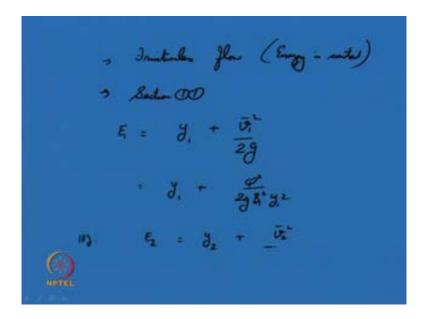
You use the same concept, again we are assuming that this is frictionless law, or total energy is constant, or the energy in the flow, energy for the flow this is constant, there is no energy loss due to friction and all, we are a assuming like that. At section 1 1 you have your specific energy E 1; E 1 is equal to y 1 plus v 1 squared by 2 g according to our formulations, this is nothing but y 1 plus Q square by 2 g B 2 square y 1 square.
