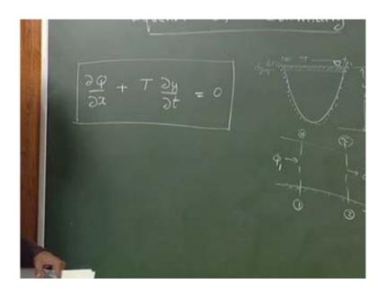
You can easily form the equation here, cancel out the repeating quantities dou q by dou x is plus dou a by dou y into dou y by dou t, this is equal to 0. Or in a most famous way, I can write the unsteady flow continuity equation as; dou q by dou x plus T into dou y by dou t is equal to 0, where t is also function of y. So, this is the famous continuity equation in unsteady fluid flow.
