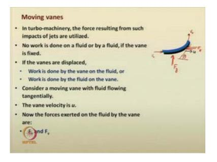
Now, we will discuss on moving vanes. How the forces are exerted on moving vanes? How we can use the same principle to analyze the moving vanes and all? So, usually, as suggested earlier also, in the turbo machinery, the force that is being resulted due to the impacts of just, jets, or the impact of vanes on the water, these are being utilized for various purposes, right.
