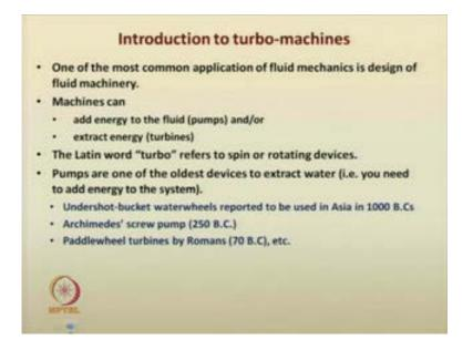
So, one of the most common application of fluid mechanics, especially in fluid mechanics and all, it is a design of fluid machinery. So, you can have various types of machines. So, machines that can add energy to the fluid flow; means, if a fluid is flowing, if you add some more energy to that, how the fluid flow occurs then? So, that types of machines are there; that is able to add energy to the system.
