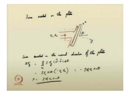
Similarly, you can now find the force exerted on the plate, force exerted on the plate, this can also be found. What could be the force exerted on the plate? Again, I am just redrawing them. Jet is coming like this, and you have the axial directions shown like this, x and y.
