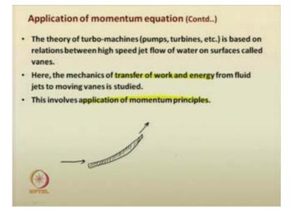
So, the same momentum equation; let us try to elaborate it. The theory of the turbo machines that is pumps, is based on the relationships between high speed jet flow of water on surface called vanes. What we want to suggest? In the previous case, we wrote this momentum equation. How we are now going to apply it for turbo machines? For that, you need to understand the theory.
