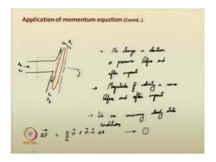
So, your equation now look like the following form. Sigma F is equal to surface integral v rho, v dot n d A. So, in that control volume given to you, you can apply this particular equation at all the control surfaces, right. This is the surface integral phenomenon. So, what are this, means, the control surfaces. You have the control surfaces; at this portion that allows water, at this portion that allows water, as well as at this particular portion where water is being allowed to transmit.
