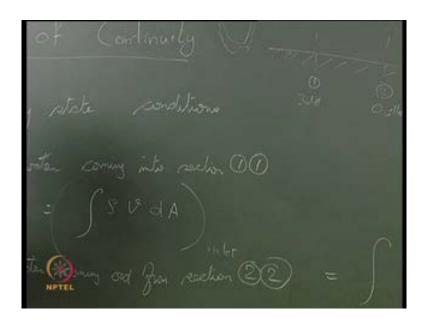
You will see that mass of water that is coming in, or mass of water that is coming out from section 2 2, is same as mass of water that is coming into the section 1 1, so we will be proceeding with the same analogy here. I can write mass of water say in this particular case, you just take any elemental strip at depth y from the free surface, and here also you can take of course, both the y is are different, this is y at the section 1 1 that you can define it as inlet.
