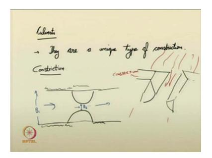
Culvert – if you look there culverts; they are a unique type of constriction. What is meant by constriction? The word constriction – what do you understand from this particular word? That is the path of the flow or the flow of water in a channel or in a river – they
