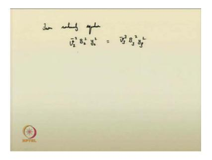
I can form a particular relationship now from the continuity equation. And, in the next class, we will derive or we will suggest the relationship of a particular parameter for the obstruction. From continuity equation, I can just suggest now, by squaring the terms B 2 y 2 square is equal to v 3 cube B 3 square y 3 square; like this. So, just incorporate the Froude number and we will see. We will get a particular relationship. We will continue regarding this portion in the next class.
