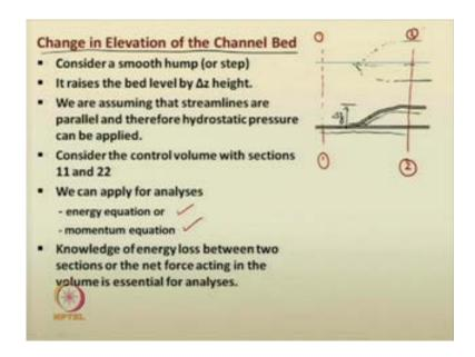
First, we will go for change in elevation of the channel bed. You see here; there is a channel bed; it has increased now towards this location; say, let this height be delta z. So, initially the water was slowing, at this level. Now, due to encountering of this raise in
