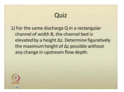
Let us do some, 2 quiz problems quickly. The first question for today's lecture is: For the same discharge Q in a rectangular channel of width B, the channel bed is elevated by a height del z. Determine figuratively the maximum height of del z possible without any change in the upstream flow depth. You have to solve it using figure; you have to explain it through figure.
