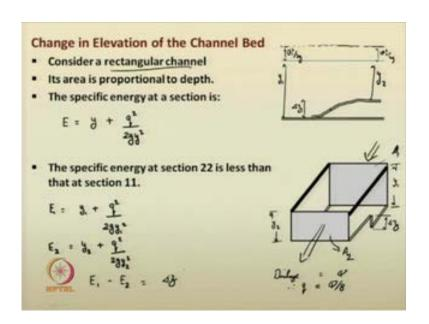
So, as we mentioned for a general channel, consider a rectangular channel, as given here, in the 2 portions. So, here, this is the upstream side; flow occurs from this direction to this direction like this. Here, the height of the section, it is y 1, and here, it is y 2, fine. There is a change in bed elevation; this height is given as del z, similarly, I can give it here also.
