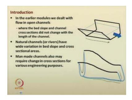
So, today is the first lecture on this particular module. So, if you look back into the previous modules, what did we observe, that is, related to the channel bed and the channel width as cross sectional width and all, you have seen that the prismatic nature; means, in most of our analysis, we have followed the prismatic nature or the prismatic section; it is being carried forward.
