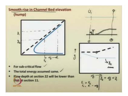
So, I can just plot it. For the smooth raise in the channel bed elevation; as this is the subcritical flow, we are assuming the total energy at section 1 1 and section 2 2, they are
