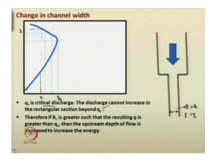
So, q c will become the critical discharge in such situations. The discharge cannot increase in the rectangular section beyond the q c value, so q c. Therefore, if B c is greater than, greater, such that the resulting q is greater than q c, if your B, if the B, constricted width B, if it is greater than B c, so that the q becomes greater than q c; that is not theoretically possible. What happens is, the upstream depth of flow is increased to increase the energy.
