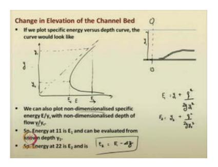
Just go through this thing. If I, if I draw specific energy versus depth of flow curve; so, these things we have done it in our module one also. So, this is a 45 degree line, where both the specific energy and depth of flow are same. So, you recall that. You know that the specific energy versus depth of flow curve looks something of this nature, and you also know that the location of the minimum specific energy E c, that is the critical energy and the corresponding depth is the critical depth.
