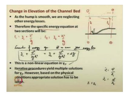
Let us assume that; here, we are suggesting the hump to be very smooth, in this case. In these two sections, the hump is very smooth. So, therefore, the energy between the 2 sections, we are assuming them, that the loss in the energy is not that much significant. Let us assume; in that way, we are trying to progress the analysis.
