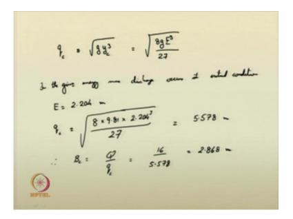
Based on this quantity, we have suggested that the critical, the given energy, given depth or given discharge per unit width, it will be having; that means, it will be having critical
