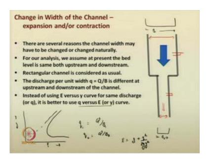
Here, just I had given a brief top view, where the channel; flow from a wider channel is occurring, flow from a wider channel is occurring and it is getting constricted within a narrow channel. So, flow is entering through a wider channel, but it is going out through a narrow channel. So, all of a sudden, there is a constriction occurring in the rectangular channel. So, how the flow is getting affected? So, these things also one need to study.
