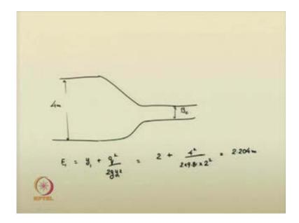
Now, you can evaluate at the; say, if the channel is getting restricted; so, here the channel width is 4 meter; this is the critical width, we do not know, what is that value B c. So, you have E 1 is equal to, at the upstream section, y 1 plus q square by 2 g y 1 square. So, I can write this as, 2 plus 4 square by twice 9.81 into y 1 is 2 square, so you just calculate it; it will come to be around 2.204 meter.
