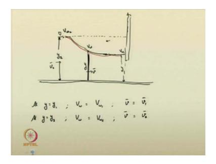
As the sluice gate is, this was theoriginal depth of flow. This is the original depth of flow in the channel. So, the sluice gate is raised like this. When it was raised the water dipped to this location and the negative surge is propagated after a few second. This negative surge reached here like that it goes on. This is how the propagation of surge occurs. So, in this case just take as we are referring any moving this thing.
