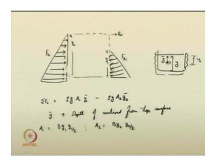
So, the net force say in this control volume now will be, such that here you have the hydrostatic force on these walls. You have the hydrostatic force on these walls like this. So, this is F p 1, the force will be in this direction I will just rube it again. So, here the hydrostatic force is in this direction. So, this is F p 2 F p 1 the weight as we are considering horizontal channels, the weight effect of weight and all that is being neglected here.
