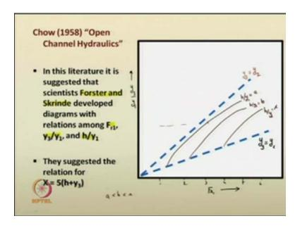
So, from Vent Chow's book on open channel hydraulics he has suggested the some of the literature works in which certain relationships of Froude number with respect to the other non dimensional numbers were given that can be used for the design purpose, especially for control of jumps by abrupt rise in the section.
