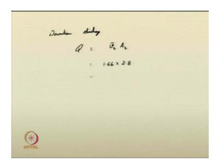
Similarly, downstream discharge increased discharge Q, you will get it as v 2 bar into A 2, by multiplying this I think I there is no need to for me to do this thing, because you already got this thing. So, two point, A 2 is 2.8, substitute this you will get the modified discharge. So, that way we would like to conclude the following portion. We will continue with this topic in the next class also.
