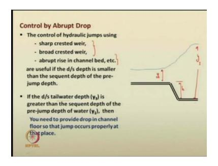
Next, which we would like to deal is the next topic which we are interested is control of jump by abrupt drops as we have studied in the abrupt rise case. Similarly, abrupt drop cases are also used for controlling various hydraulic jump for example, just recall the things in the sharp crested weir, broad crested weir as well as the abrupt rise in channel bed. What were the situations that for which all situations you used these mechanisms to
