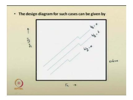
May I beg pardon I just forgot to mention; you can also device design curves for abrupt the control of hydraulics, control of jumps by hydraulic jumps by drops. So, here also we can say for the incoming flow Froude number, or the pre jump Froude number ratio y 3 by y 1 for the various cases say h by y 1 is equal to a h by y 1 is equal to b h by y 1 equal to c for different values of this particular ratio h by y 1 a b c where a is greater than b it is greater than c like that.
