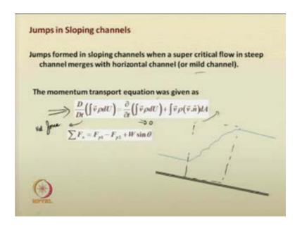
So, in the jumps in the sloping channels, if you recall them, it is a form when a supercritical flow from steep channel merges with horizontal channel, or in the files or it can be a mild channel also. The momentum transport equation was given for a control volume, right. If you recall them, the control was specified, and momentum transport equation was given in the following form.
