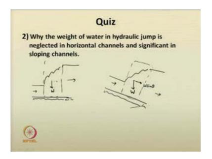
Next question we had asked was: Why the weight of water in hydraulic jump is neglected in horizontal channels, while it is significant in sloping channels. So, you just need to draw the figure horizontal, horizontal channel jump occurring there; just show that in the hydraulic jump the weight of water is acting vertically downwards, the flow is horizontal. So, there is no component of weight in the flow direction.
