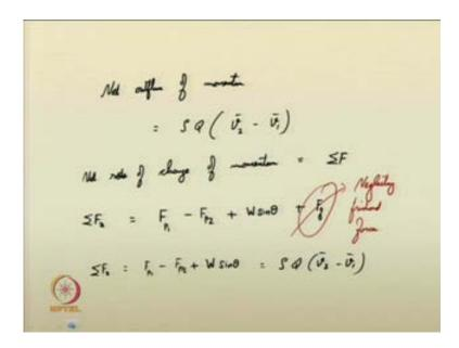
So, I can write, the net outflux of momentum, net outflux of momentum through the control surfaces is nothing but, rho into discharge into, v 2 minus v 1 bar. The net rate of change of momentum is equal to the change of, rate of change of momentum is equal to the net force in the control volume.
