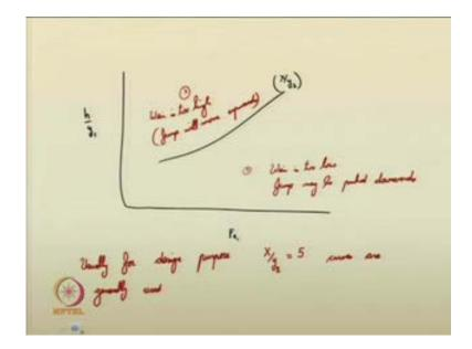
So, again, I am just redrawing the thing here. You can see that, as this is froude number, this is h by y 1 number, and this is the curve for any particular value of X by y 2 ratio. So, in this case, you have, say, points lying above this particular line of x by y 2, you have points lying below, and also on the right of this X by y 2 curve. So, you can have 2 different situations. What does this infer?
