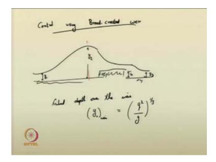
So, applying the conservation, means, was specific energy theorem, just say in this particular situations; say, may be in this following sections.
