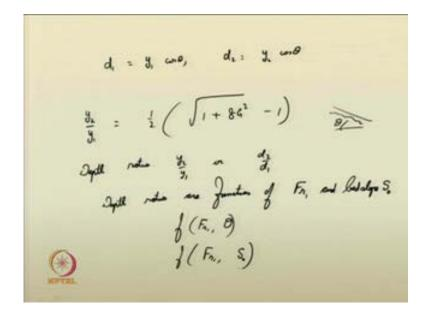
As d 1 is equal to y 1 cos theta, d 2 is equal to y 2 cos theta, the above relationship can be changed to vertical depth, y 2 minus y 1 is equal to half of, root of 1 plus 8 G square minus 1, right. So, you are getting the depth ratios, y 2 by y 1, or d 2 by d 1.
