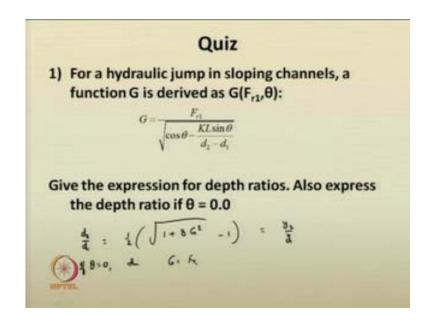
So, the solutions for this case are, you have the depth ratios d 2 by d 1 is equal to half of, root of 1 plus 8 G square minus 1. This is same as the vertical depth ratio, y 2 by y 1 also, right. This is how the depth ratio expression is given to you. So, if theta is equal to 0, then what happens? G is equal to F r 1 itself. So, you will get the depth ratio y 2 by y 1 appropriately.
