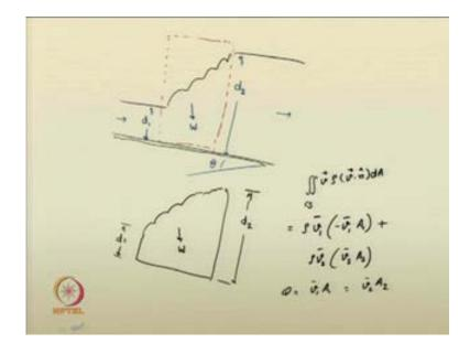
So, as we can see it from a side section, the jump, the weight of the water is significant, as you can see it here. I am just describing a control volume given in the red color here. So, that control volume, if you take into account; so, the control surfaces, I am just taking the control volume. So, here you have depth d 1, here you have depth d 2, right; and, there is weight of water acting downwards.
