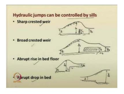
Next, we will discuss on control of jumps. Hydraulic; as we have studied earlier, hydraulic jumps require some certain control, so that it will be held within that stilling basin. Otherwise, you have seen how it can be pushed in the upstream, or it can be pushed downstream, or it can get washed away; so, there various provisions of controlling the hydraulic jumps.
