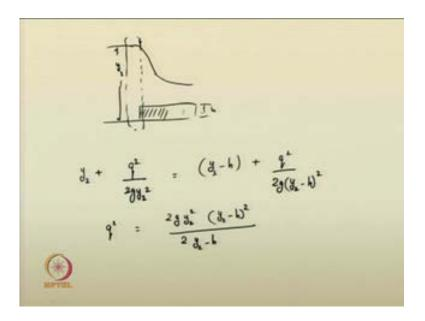
So, using the specific energy at equation for the 2 sections; say, this is your broad crested weir of height h. Then, this is where the jump is coming now. So, for these 2 sections, in these 2 sections, we can suggest; say, here this is y 2. So, between these 2 sections, the energy equation will look like this: y 2 plus q square by 2 g y 2 square is equal to; so, here this is y 2 minus h, y 2 minus h plus, q square by 2 g y 2 minus h whole square.
