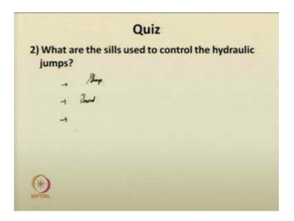
For the next question: What are the sills used to control hydraulic jumps? So, you know the solution for that; broad sharp crested, broad crested, then abrupt rise, abrupt, abrupt rise in the bed, abrupt, lowering of the bed. So, these are the answers for the second question.
