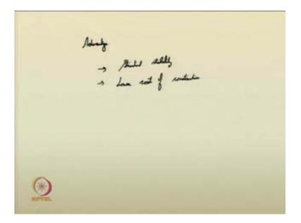
What is the advantage of broad crested weir, advantage of broad crested weir? So, broad crested, they are structurally stable, structural stability and lower cost of construction compared to abrupt rise. So, for these cases, you use broad crested weir. So, that way I was thinking of continuing the other 2 cases of controls; but, however due to time limit we will continue it in the next class. We will have a quick quiz related to the following topic.
