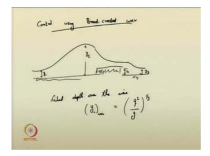
Next, we will see control; there is the, again the control of jump using broad crested weir. So, you have a broad crested weir for the jump. So, you can have different tailwater depth, let us see; again, this is the prejump depth, this is the sequent depth of the prejump, this is the height of the sill, and here let us assume y 3 as the tailwater depth.
