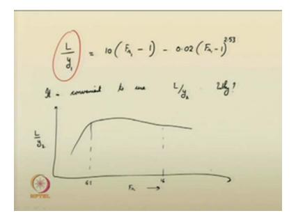
They suggested that the ratio of length of the jump with respect to its pre jump depth. This can be given as 10 times Froude number in the upstream or the pre jump location minus 0.02 times Froude number minus 1 to the power of 2.53. So, if you have this, this was one relationship, they have developed empirically from their experimental data. You can see that this ratio was obtained by using the length of the jump with respect with the pre jump depth, but mostly it is convenient.
