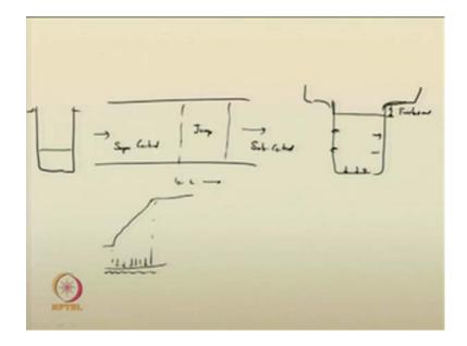
So, if there is a, channel water is flowing, say here it is in supercritical and at this location you are providing the location for jump and say if this is the length of the jump and from here it is subcritical. This is the top view of a in a channel where jump is occurring. So, when you design the channel in this case, say if the channel cross section, if that channel cross section you had the depth of flow like this, here the depth of flow as this particular quantity.
