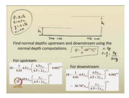
So, we are given that Q is equal to 18 meter cube per second, width is 4.5 meter. Therefore, discharge per unit width is equal to 18 divided by 4.5 4 meter per second. This was seen in the last class also similar case. So, let us consider this as steep slope channel and this portion as mild slope channel. This is having 0.002; this is having 0.001, here the normal depth is y n 1 and here the normal depth is y n 2.
