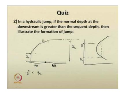
Second question; "In a hydraulic jump, if the normal depth at the downstream is greater than the sequent depth, then illustrate the formation of the jump." You have to figuratively illustrate that; I am not asking you in a mathematical formula. You can illustrate that; you can just figuratively explain solutions for this quiz.
