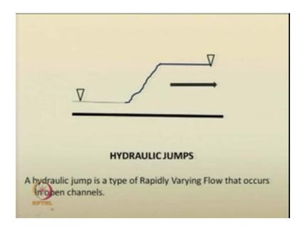
Welcome back to our lecture series on advanced hydraulics. So, we are in the fourth module on hydraulic jumps. If you recall them hydraulic jumps, it is a type of rapidly varying flow that occurs in open channels.
