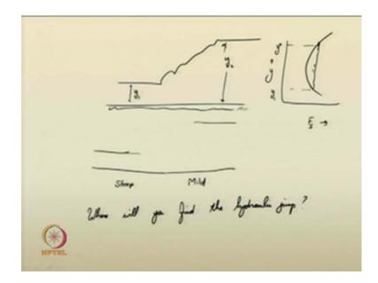
So, when we studied the hydraulic jump, you have already seen that the hydraulic jump consist of a pre jump depth and a post jump depth, we have seen these things. So, the specific force in the pre jump location and the post jump location, they are the same. Also for rectangular channels and all in our previous analysis and all we have approximated the bed channel to be almost horizontal and all.
