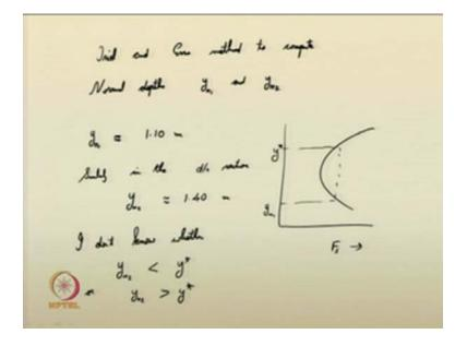
You can use trial and error method. So, you can use trial and error method to compute normal depths y n 1 and y n 2. So, once you compute the normal depths based on the given data I have observed that normal depth in the upstream portion it is approximately equal to 1.10 meter, it may be 1.095 meter and all. But I am just taking at the 2 decimal level.
