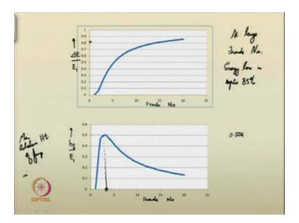
So, using this relationship we had developed this particular curve. The second curve, the second curve is related to again Froude number in the x axis and the relative height. We have already mentioned that the relative height h f by E 1 quantity on the x or y axis. So, this quantity also again we can suggest it in the following form. You will see that the
