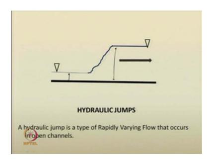
If you recall hydraulic jump means, it is a type of rapidly varying flow, where the depth of flow suddenly increases from a low depth to a greater depth. These things we are discussed it in the last class.
