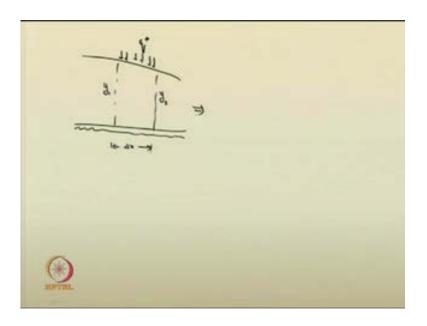
So based on that thing, I can just suggest now, the following thing. This is the bed slope; let this be the depth y 1 at section 1 1; y 2 at section 2 2; they are separated by a del x; this is the control volume, earlier we suggested; we are having an increasing discharge at rate q star per unit length, having flow.
