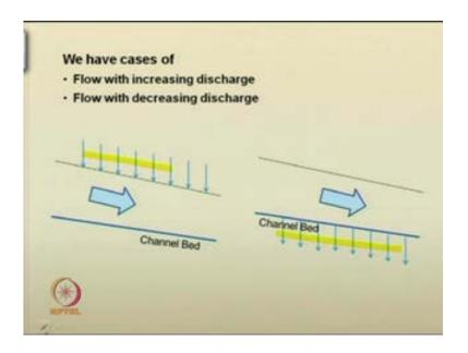
We have seen that, there are two types of spatially varied flow; that is, flow with increasing discharge; in the reach, in the flow, if the channel flow is in this direction and
