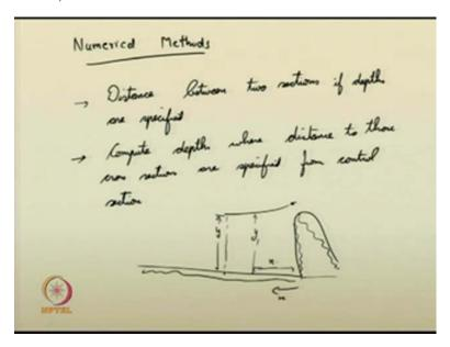
So, the most important method, which we hereafter will be always referring is the numerical methods; the idea behind numerical methods. Numerical method, it is an approximate method for solving differential equation. It is not the direct method, whichever you have studied in your high school levels or in your college levels and all, the numerical method does not follow the direct approach. It is an approximate approach.
