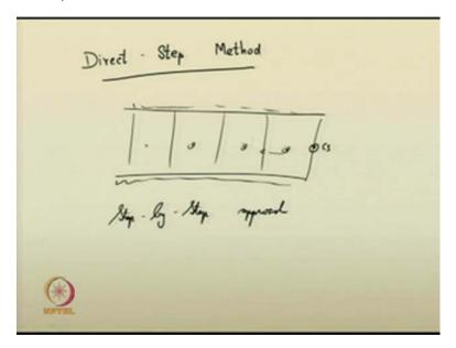
The first method which we are going to do is, direct step method. The first method is direct step method. What you are going to do is, the channel reach, whichever channel reach is there; say, if there is an obstruction and gradually varied flow profile is there, it is, the channel reach is now divided into short reaches. You will compute the properties now, in each of the small reaches, then you club them.
