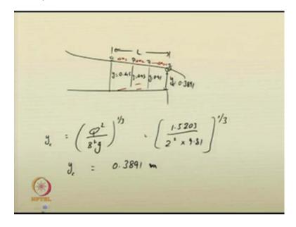
Now, before that, let me suggest to you, the same discharge at the brink; say, at the brink, here the depth will be critical depth. So, the critical depth, you can easily compute for the rectangular channel as B square g power of 1 by 3. Substitute the values, 1.5203 by 2 square into 9.81 whole to the power of 1 by 3. So, your critical depth is observed to be 0.3891 meters, ok. So, the critical depth for the flow is 0.3891. So, at the brink the depth is 0.3891.
