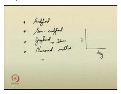
In general, to solve a differential equation, the various methods- you have analytical methods, you can also use graphical methods, and the most common and widely used method is the numerical methods. So, you can use any of these methods to solve the differential equation, that is the dynamic equation for gradually varied flow.
