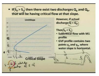
If your bed slope is greater than the limit slope, then; let us see that, how you can demonstrate? This is your limit slope. So, if your bed slope is greater than, say, let this be your bed slope S 0, if this is greater than the limit slope, then you can observe easily 2 discharges; say, this is discharge, I can write it as Q a, and this is discharge Q b. That is, for the same bed slope S 0, for
