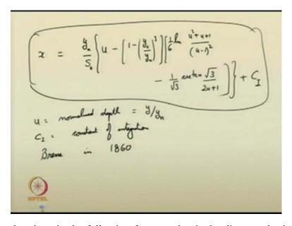
If the solution can be given in the following form: x, that is the distance; horizontal distance x, this is equal to y n by S 0 into, u minus, 1 minus, y c by y n whole cube into, 1 by 6th of natural
