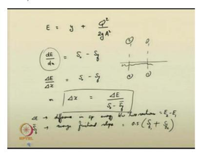
Just recall your specific energy equation, y plus Q square by 2 g A square. So, the direct step method, we can use mostly for the prismatic sections only. For non prismatic sections, this method is not that convenient. So, we will see it later. So, please note that this, how you are going to use them?
