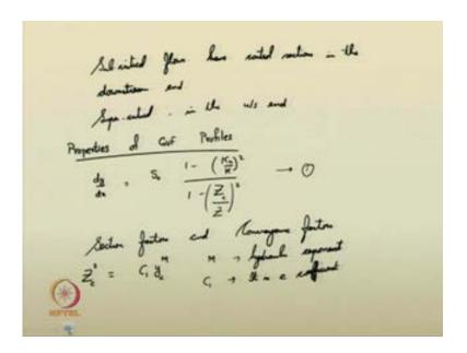
We have to note that, usually, the subcritical flows have control sections at the downstream of the profile; that is, the subcritical flows have control points in the downstream end as you have seen in the spill way example, say in the previous slide for the... Say this is the M 1 profile; it starts somewhere here and it goes like this. But the
