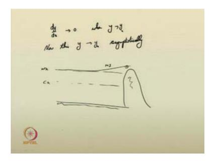
As we mentioned earlier, dy by dx tends to 0 when y tends to y n. Now, this y tends to y n is possible or it reaches or becomes y n asymptotically. So, you will require a very large length. Say if you are starting say in this particular case, you have such an obstruction dam, critical depth line, normal depth line. And if you want to compute the M 1 profile, this M 1 – this gradually varied flow profile reaches the normal depth
