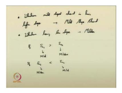
That is whichever mild slope channel is having higher slope it is called mild slope channel and whichever is having less slope; the magnitude of the slope if it is less they are called milder slope channels. So, say, if S 01 greater than S 02 then this is milder slope channel; may I beg your pardon? S 01 greater than S 02; this is mild slope channel and this is channel 2 is milder slope. Similarly if S 01 is less than S 02, then channel 1 is
