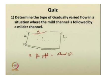
The first question it is very simple and straight forward you are asked to determine the flow profile. So, it is a situation where a mild channel followed by a further milder channel. So, you have the critical depth same for both; the normal depth in mild channel
