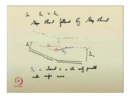
And for S 0 1 greater than S 0 2; so for S 0 1 greater than S 0 2, it is having a steeper channel followed by steep channel. So, in this case a steeper channel followed by a steep channel. So, you have the normal depth line like this. Here the normal depth line is like this, the critical depth lines will be like. This is your y n 1 and this is your y n 2. The only
