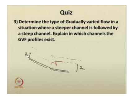
So, the next question asked was GVF in a steeper channel followed by a steep channel, a steeper channel followed by a steep channel. So, you have your critical depths like this. You have here the normal depth is somewhat like this; here the normal depth is y n 2 greater than y n 1. So, the possible curve is an S 3 curve; S 3 is the only possible gradually varied flow profile for such a situation. So, this is the way.
