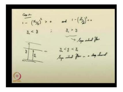
Let us consider the case 1. The case 1 is say, 1 minus k n by k whole square – how did I write the in the last slide? That is, 1 minus k n by k whole square greater than 0; and 1 minus z c by z whole square should be less than 0. What does that this mean? So, k n by
