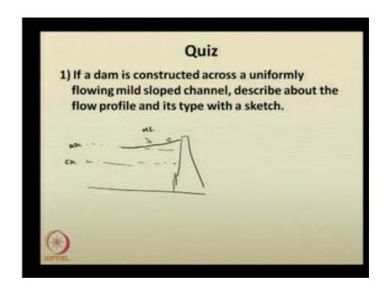
The solutions for today's quiz; you can see that, if a dam is constructed in a mild sloped channel, normal depth... This is your critical depth line. In the upstream of the dam, you will see the water surface profile rising like this. And this water surface profile is called M 1 water surface profile. So, this is in the mild sloped channel.
