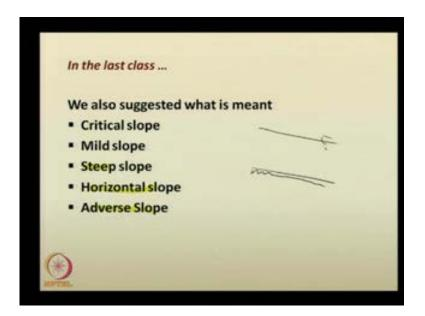
We also suggested you, what is meant by critical slope; that is regarding the bed slope of the channel. If you recall the bed slope of the channel; for any channel, the bed slope – it can be considered as a critical slope; it can be considered as a mild slope; also, it can be considered as a steep slope, horizontal slope, adverse slope. All this things we have described it in the last class.
