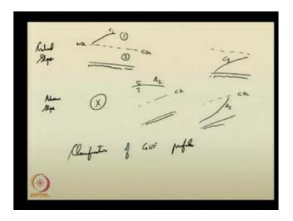
Do I need to describe it here? I will just briefly show it again. For the critically sloped channel, you have both the critical depth line and normal depth line as the same; both are
