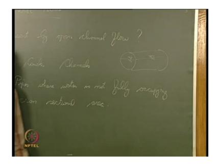
And if the level of water is only this much and it is open to atmosphere, if the top surface of water, if it is open to atmosphere even in these closed pipes the flow is called open channel flow. It does not matter if it is an enclosed conduit and all if, is if the top surface of water is open to atmosphere it is considered as open channel flow. Why do you study open channel flow? What are the various proposes? Why do you want to study open channel flows?
