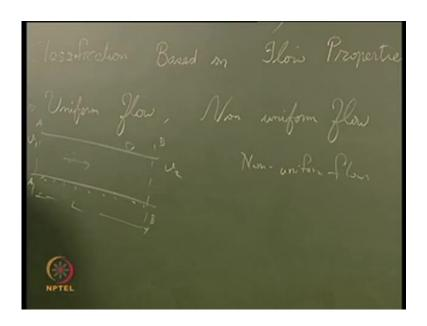
Uniform flow as the name suggests say any fluid properties velocity discharge height depth whatever be, whatever properties you are taking if these properties are uniformed for a considerable stretch of the channel, then such type of flow are called uniform flow. Say if a channel stretch of length l if it is taken and if it is found that this velocity v from section A A to section B B, if it is having the same velocity throughout this length then that is called uniform flow.
