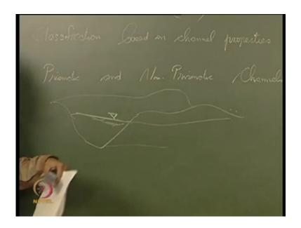
For example, a river cross section, a natural drain cross section and all they are the cross sectional area the width of the channel depth of the channel. They are all vary with distance, so they are called classified as non prismatic channels. Our next classification based on channel properties they are natural and artificial channels.
