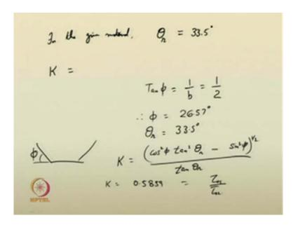
For the given material, it is observed that your angle of repose is equal to 33.5 degrees. If you have this particular data 33.5 degrees, then well you can easily find what is the tractive force ratio now? Because this phi is already known to you, this angle phi is already known to you, because tan phi is equal to 1 by B is equal to 1 by 2. Therefore, phi is equal to 26.57 degrees theta r is also given to you 33.5 degrees.
