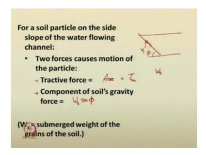
So, for a soil particle on the side slope of the water flowing channel two forces causes motion of the particle that is the tractive force. So, tractive force, how can I write it? It is nothing but the area where the tractive force is there into the quantity tractive force.
