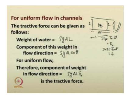
So, as we mentioned so the weight of water again for your convenience I am just drawing it. So, if the channels is having a slope, slope this is equal to tan theta. So, that slope of the channel it can be a given as the bed slope S 0 then the weight w is acting here and the weight of the water. Now, if this length if this length is L, then you know that this is nothing but density into acceleration due to gravity into area of cross section
