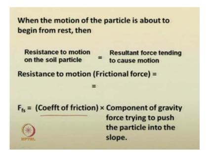
So, when the motion of the particle is about to begin from the rest. It is the simple mechanics principle when the motion of the particle is about to begin from rest. Then the resistance to motion on the soil particle is same as the resultant force tending to cause the motion.
