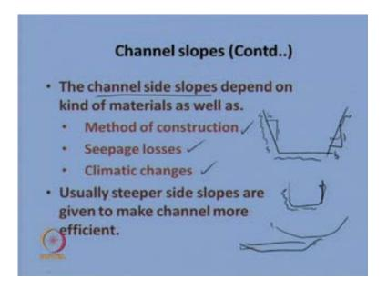
So, in the channels slopes, we suggested that the channel side slopes are also quite important. The channel side slopes, it depends on the various kinds of materials, you have seen that. You can use different types of materials for construction of channels. So, based on the materials, one may have to adopt the sides slopes; say here, in the side slope, what should be this ratio, 1 is to b, this ratio 1 is to b is are the side slope.
