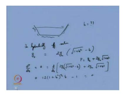
The solution for this particular problem as suggested. So, this is the trapezoidal section; we have asked you, means we have already seen that for hydraulically efficient section your B naught, or the channel bottom width should be equal to twice the normal depth into root of 1 plus b square minus b.
