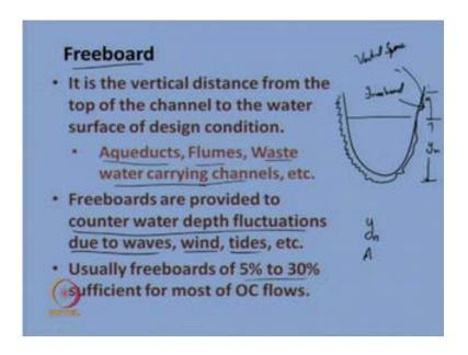
The next design factor while designing the non erodible channels mentioned was freeboard. What is meant by freeboard? Just consider a channel section; in the channel cross section, you have designed, means, using the various design criteria parameters you have designed that, say, the depth loop, y n should be so and so. Then you suggested that the area of flow should be so and so.
