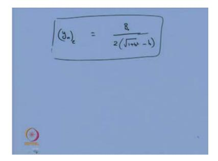
You can also see that, or the hydraulically efficient channel cross section, the normal depth should be equal to B 0 by twice root of 1 plus b square minus b. So, this relationship has to be followed. So, you can use this thing; as seen in the rectangular cross section, the hydraulically efficient cross section, the depth of the normal flow should be equal to the half of the width of the channel. Similarly, here, this is B 0 by 2 into certain quantity, root of 1 plus b square minus b.
