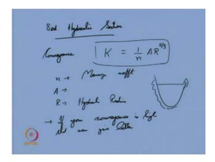
So, the next portion which we are going to discuss is the best hydraulics section. So, what is meant by best hydraulic section? If you recall the term conveyance; I hope you recall them, conveyance K, for uniform flow it was given as, according to Manning, from the Manning's equation 1 by n A R to the power of 2 by 3, where your n is Manning's coefficient, roughness coefficient; A is area of cross section; R is your hydraulic radius.
