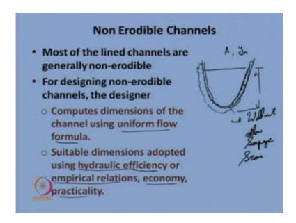
Then non erodible channels. So, most of the lined channels, most of the channels which are lined, for example, if you have any arbitrary cross section of the channel, if this is channel bed, and if you line the channel bed with some material, such channels are called lined channels. So, they allow, means they would not allow, will not allow seepage, or will not allow scouring along the bed; along the bed it will not allow. So, such lined channels are generally called non erodible channels.
