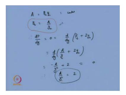
If A is equal to B 0 y n, equal to constant; that means, your B 0 is nothing but A by y n. Therefore, d P by d y equal to 0 means, d by d y of B 0 plus 2 y n; this is d by d y of A by y n plus 2 y n. What is this quantity? A is a constant, we suggested A, all through design already A has been established; A is a constant. So, it is not going to vary.
