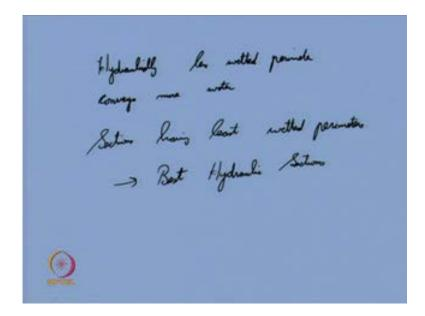
So, hydraulically, so in terms of hydraulics, or hydraulically less wetted perimeter conveys more water fine. So, you can say that the sections having least wetted perimeter, such sections are called, sections having least wetted perimeters, they are called best hydraulics sections.
