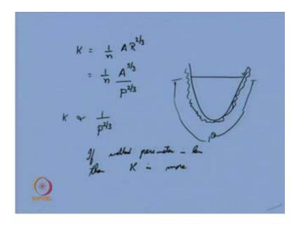
So, for your conveyance factor, K is equal to 1 by n A R to the power of 2 by 3, this is 1 by n A to the power of 5 by 3, P to the power of 2 by 3, fine. So, whatever wetted perimeter you have, whatever wetted perimeter you have for the cross section, you are seeing that the conveyance is inversely proportional to P to the power of 2 by 3. So, if your wetted perimeter, if it is less, if wetted perimeter is less, then K is more, your conveyance is more.
