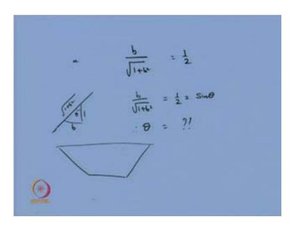
So, you know, for the slide slope, we are talking about the side slope of the channel, 1 is to b. So, root of 1 plus b square, it indicates your hypotenuse of this portion. So, what does this mean? So, this, if you note about this angle as theta, so you can easily suggest that, b by root of 1 plus b square, is equal to half, is equal to your sine theta; therefore, what is theta? That is quite obvious to you. So, I am not going to discuss further. So, if
