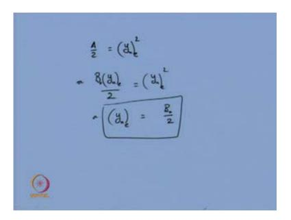
So, you will see that, you will get B 0 y n into e, by 2, is equal to y n the whole square; or, it suggest that; so this is the criteria for the most efficient, hydraulic efficient, or the hydraulically efficient rectangular cross section; that is your depth of flow should be half of the width of the channel. So, that is the criteria. So, here the suffix e is showing the hydraulically efficient channel. So, for rectangular channel, one can prepare it like that.
