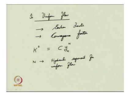
In uniform flow, you have already seen section factor, conveyance factor. So in uniform flow also, the conveyance factor now can be given as K square is equal to some
