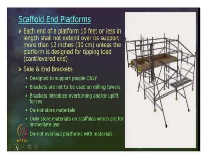
Now the scaffold end platform as a cantilever should not be loaded up and use like a cantilever means. Unless it is specifically designed for tipping load which is primarily the cantilever action unless it is specifically designed and recommended. It should not be used as a normal platform the side and end brackets designed to support people only and not for equipment. And for other, only for inspections for checking something people can use but not for loading and storage of materials.
