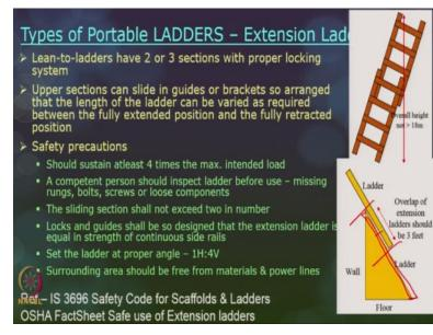
The next type of portable ladder is extension ladder as the name implies there can be 2 or 3 sections of the ladder which can be together. And you can have a adequate guides or brackets set up so that it can slide in and out in order to do a different reach of the levels. You can vary the
