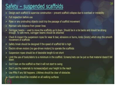
Now, we will talk about the safety precautions again as I told all scaffolds should be designed, constructed, erected under the supervision of a skilled person. And you should do proper care while you are designing and constructing these scaffolds. Design each scaffold and supervise to prevent scaffold collapse due to overlap load or instability. And there should be a competent person to do full inspection before using the scaffold.
