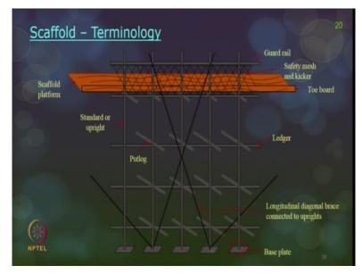
If you see some pictures of this scaffold, these are the pictures and all the parts are all labeled here. And if you see here if the scaffold platform is not stable you can also have an base plate so that this scaffold are firmly put in place.
