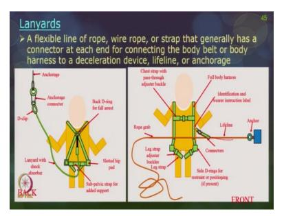
Again, there are so many types of lanyards like for example single leg lanyard and double leg lanyard, shock absorbing lanyard and so on. Single leg lanyard means from the worker you have single point of anchorage, double leg lanyard is from the worker you have 2 points of anchorage. So double leg lanyard is considered more safer in terms of protection than a single leg lanyard.
