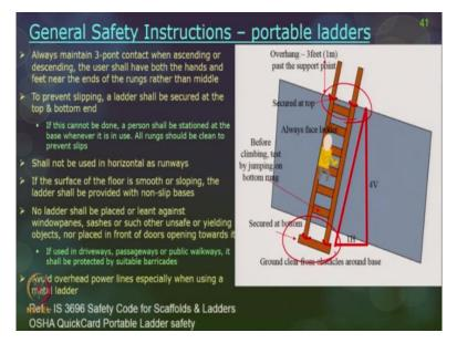
Now general, safety instructions for any portable ladders always maintain a 3-point contact when you are ascending or descending a ladder. So, the 3-point contact is either 2 hands and 1 leg on to the rungs so primarily you have to put the 2 hands on to the side rails and both the legs on to your rungs. And these 2 hands should be closer to the side rails on the rungs or on the side rails and feet also should be closer to the side rails only even though it is on the rungs.
