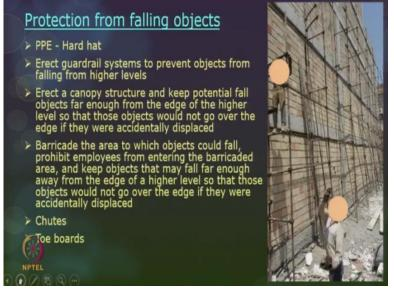
Next protection from falling objects, so PPE is compulsory, try to wear hard hat when you are passing by place where this is a hazard of falling objects. Erect guards, rails system along with the debris net so that objects are not falling from higher levels. Erect a canopy structures there is a public path way or something it is better to have a canopy structure. So that these falling objects are not, on to the public or to the workers who are passing below the site?
