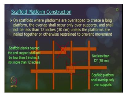
Scaffold platform now let us talk about the platform. So, the platforms should not be when the platforms are to be overlapped in order to have a very long length of the scaffold. So, they can be overlapped only on the supports and this overlap should not be less than 12 inches or 30 centimeters in width. And this should happen only along the supports and not on the middle of the support.
