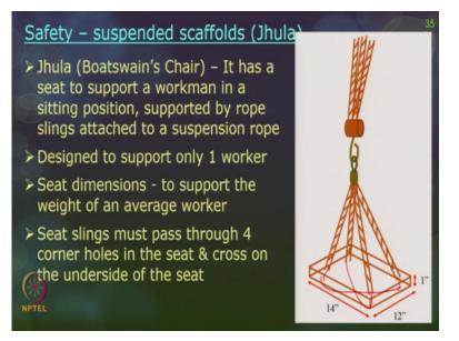
And as I told there is 1 separate suspended scaffold which we will discuss and aerial lifts safety we are not covering in this course. So can suspended scaffold is special variety of suspended scaffold called Jhula which is also called Boatswain's Chair which is primarily designed for one worker to sit and finish his work. It has a seat to support a workman in sitting position and supported by rope slings attached to a suspension rope.
