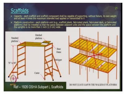
Now let us talk about each and every part of the scaffold and what does the safety requirements talk about. So, scaffolds capacity each scaffold or its scaffold component should be capable of supporting without any failure at least 4 times the maximum intended load. If you plan for a load x it should be at least able to accept 4x the load. And platform construction so each platform unit
