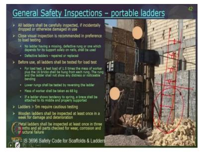
So general more safety precautions on portable ladders. So, all ladders should be carefully inspected if incidentally dropped or damaged and other wise used it should be inspected before usage. Close visual inspection is recommended even more than a load testing. So, no ladder having a missing or defective run or which depends on support only on nails or something should not be used.
