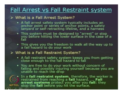
So, this fall arrest system and fall restrain system let us discuss little bit so both these systems generally have PFAs as a back bone. In a fall arrest system, they are deigned to arrest or stop few before hitting the lower surface in the case of a fall. So, it is like we will not fall. It is like a dog and leash. So, with the leash the dogs can move only till the leash length same way it is nothing but a fall arrest system we will not go beyond the certain limit and try to fall.
