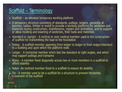
So, in general if you see this scaffold terminology, it is nothing but an elevated temporary working platform for enabling the workers to climb up on to the and reach the working place and this is temporary structure which consist of standards, put logs, ledgers and generally of bamboo or timber or even metal aluminium. There are so many scaffold materials, as come in place and also we have customized scaffold as well as commercially available manufactures scaffold also available these days.
