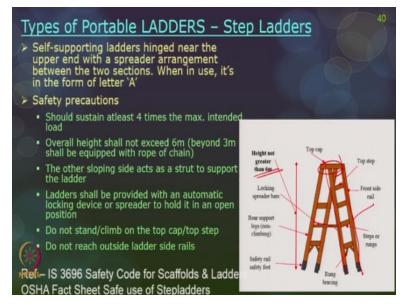
The next type of portable ladder is step ladder this is also called as A ladder because it as a shape of A when in full expanded position. So, self-supporting ladder hinged near the upper end. The upper end is actually close together with the spreader arrangement between the 2 sections when in proper use its actually looks like A letter and that is where it is also called A ladder. Safety precautions again this ladder should also be able to sustain at least 4 times a maximum intended load.
