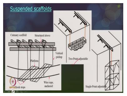
Then 2-point adjustable, single point adjustable and you also have catenary scaffolds. So, most of the safety precautions which; I am going to talk about in this suspended scaffold will be easily fitting in for 2-point adjustable scaffolds.
