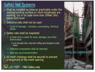
Next, we will talk about safety nets so this is again when you talk about for protection safety nets is one of the ways to safe guard people from falls. So, what is the safety net? So, this safety nets are primarily to catch worker or people from when they fallen down. So, this should be installed as close as possible under practicable under the walking or working surface from where employees are expected to fall.
