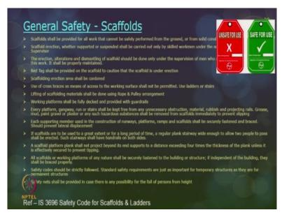
General safety again a recap on the scaffolds that, we have talked so far. Scaffold shall be provided for all work that cannot be safely performed on the ground or from solid construction works. So, scaffold erection whether suspended or supported shall be carried only by skilled workmen or by a competent authority under the guidance of a supervisor. The erection alterations dismantling of scaffold should be done only under the supervision of a competent person.
