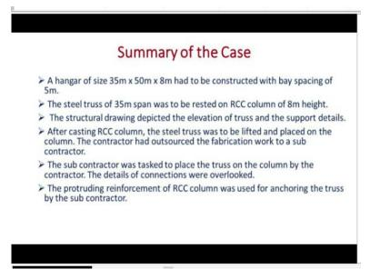
A hangar of size 35 meter by 50 meter by 8 meter high had to be constructed with a base spacing of 5 meter. The steel truss of 35 meter span was to be rested on RCC column of 8 meter height. The structural drawing depicted the elevation of the truss and the support details. After casting RCC column the steel truss was to be lifted and placed on the column. The contractor had outsourced the fabrication work to a subcontractor.
