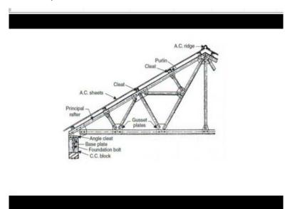
Having understood the background now we will look into the scientific reasons behind this accident and what our lab says led to this mishap. The figure shows the typical cross section of etrus with connection details. The support details include the foundation boards embedded in reinforced cement concrete and the base plate at the top of RCC column.
