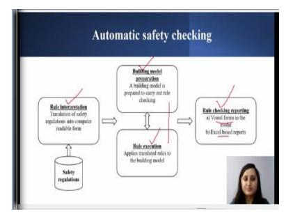
There are four components of automatic safety checking, the first one is a rule interpretation, which involves the translation of human readable set of safety regulations into the computer readable form. The second one is building model preparation, which involves building of a model wherein we have to execute the rules, the converted rules, the third one is rule execution, there we have to apply the translated rules into the building model.
