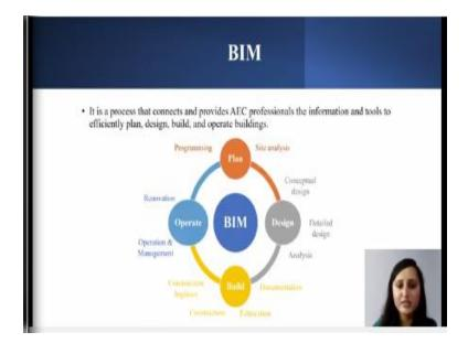
BIM is the process that connects and provides the AEC professionals with the information and tools to efficiently plan, design, build and operate buildings. So, we can say that BIM is more than just designing, it is not limited to just use in the design phase. But can be used in the entire lifecycle of the project as shown in the figure. That is, we can use it in the planning phase, designing phase, building phase, operating phase, and even the control this renovation and demolition phase.
