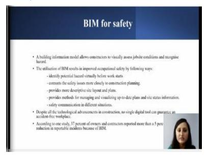
Now comes for BIM for safety, it is desirable to have a technology which may have been analyzing and communicating safety related issues. In the recent years, due to the growing application of BIM in construction industry. Researchers as well as industry professionals have started using BIM to enhance construction safety. As BIM shows a visual representation of a facility, a BIM model allows the constructors to visually assess jobsite condition and recognize hazards.
