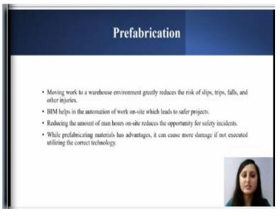
Now, let us discuss prefabrication, when we move our work to a warehouse environment, it greatly reduces the risk of hazards such as slips, trips, falls and other injuries. BIM and prefabrication have led to many favourable scenarios that help in reducing the risk. BIM helps in automating the work on site, which leads to safer projects. We can simply say that reducing the number of manhours on site reduces the chances of incidents happening on site.
