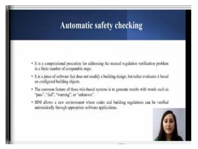
Last but not the least is automatic safety checking. It is also referred to as automated rule based checking or automated code compliance checking. As term indicates, we can understand that it has something to do with the rules or the codes. In simple terms, we can say that it is the process to automate and check against the set of rules. It is defined as the computational procedure for addressing the manual regulation, verification problem in a finite number of computed steps.
