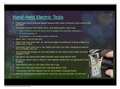
Now hand-held electrical tools, most of these construction workers use hand-held electrical devices which are generally in contact with the hand till the equipment is in usage. So, these tools pose a potential danger because they make continuous good contact with the hand. So, to protect workers from shock, burns or electrocution, these tools must have a 3-wire cord with the ground and be plugged into grounded receptacle or double insulated or powered by a low voltage isolation transformer.
