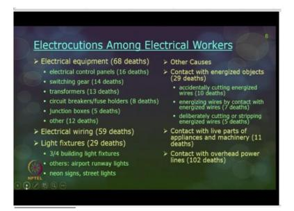
Now little detailed statistics on electrocution among electrical workers, electrical equipment 68 deaths, if you see the inner distribution, electrical control panels, switching gear, transformers, circuit breakers, junction boxes and others. Electrical wiring 59 deaths, light fixtures 29 deaths, three fourth for building light fixtures, others for airport, runway lights, neon lights, street lights and so on.
