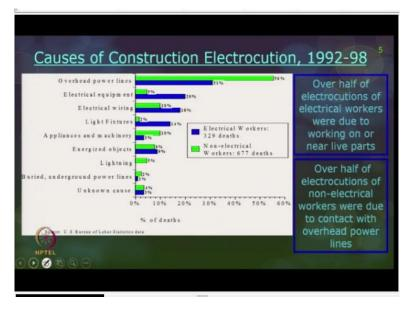
Now causes of construction electrocution. So, this is also the statistics taken for 6 years put together, overhead power lines is a number 1 of accident. This is primarily with regard to non-electrical workers, overhead power lines, then electrical equipment, electrical wiring, light fixtures, appliances and missionary, energized objects, lightning, buried underground power lines and unknown causes.
