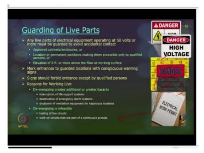
So, any live parts of electrical equipment operating at 50 volts or more must be guarded to avoid accidental contact. So, approved cabinets, enclosures all should be made, you should also mark the location and say danger, high voltage and so on or sometimes you can also move for an elevation of say 8 feet or more above the floor or working surface, so that it is not in contact with any of the workers.
