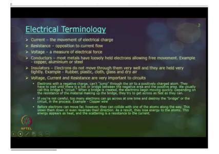
So, any material that can conduct electricity will be able to close that open circuit if the circuit is not closed properly, some of the terminology with electricity current. So, the movement of electrical charge is generally termed as current. Resistance: the opposition to current flow is called resistance. For example, suppose if you are taking an example of the garden hose which you use for watering the plants.
