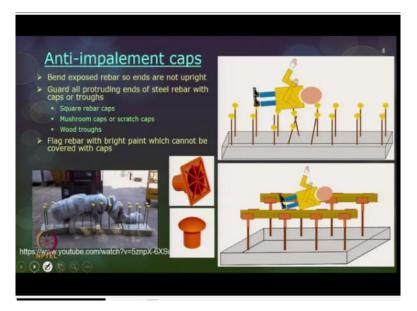
The other that is a safer way to do in sites, other method is providing an anti-impalement cap. So, bend all the exposed rebar so that the ends are not upright, it is a natural way of protection. Otherwise, you can also guard all the protruding ends of the steel reinforcement bars either by using caps or by using troughs. Caps again there are 2 types; one is your mushroom cap or the scratch caps.
