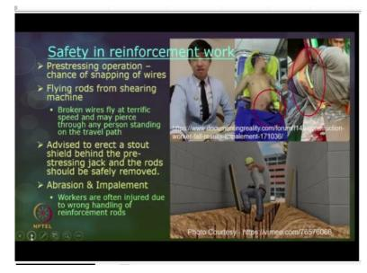
There are so many issues for example, you may do pre-stressing and post-stressing operations, wherein the reinforcement rods are actually strengthened using a pre-stressing jack. So, there the primary hazard is snapping of wires. I am not discussing all the hazards with regard to steel, but few issues I am just bringing in and primarily we will move on to welding operations only.
