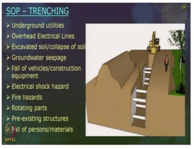
So again, what are all the different hazards available underground utilizes overhead power lines then excavated soil or collapse of soil. Ground water seepage, fall of vehicles fall of equipment fall of person. Electrical shock hazards fire hazards rotating parts of these moving machinery preexisting structures. So, these are the different hazards available.
