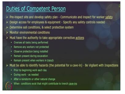
Now, duties of a competent person, so pre-inspect the site and develop a safety plan. Communicate and inspect for worker safety and design proper access for employees and for the equipment. Determine the soil condition and select a protection system whether it is sloping shielding or shoring systems. Monitor the environmental conditions for any you know rain or something happening then you should not be taking up series or severe activities.
