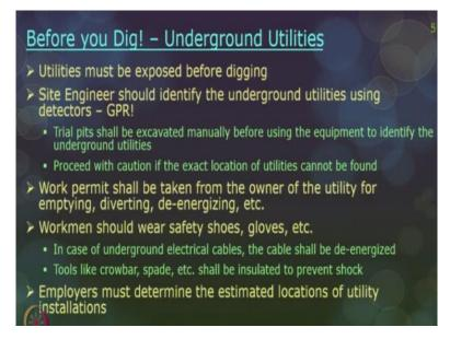
So, the next precaution so first is you have posted a message you have allowanced to the public you have given enough warning signals on excavation is going on. The second precautions, that you have to do is identify all the buried underground utilities. There are so many underground utilities which are buried inside the ground and you may have to identify all of them so that do not mess up with those utilities when you are actually putting your know excavator equipment there.
