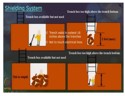
Now let us see more on the trench shields or trench boxes, some so these trench shields are like boxes they come as boxes and with which you have to put in to the excavator portion. As you start, cutting out the earth you have to put these boxes inside and the workers can actually start working inside these boxes. Now the next hazard which is seen in the construction site is water accumulations.
