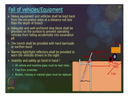
For fall of vehicles or equipment before that so this is ladder which I talked to you in the last slide. So at least 1 meter above the ladder has to extend this is primarily for workers to climb or escape in terms of an emergency. The heavy equipment and vehicles shall be kept back from their excavator sites at a distance of not less than the left of the trench. So, they should be really away from the excavated site and adequate and well anchored chop block.
