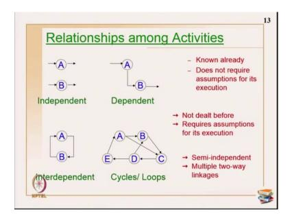
So, now as I explained verbally I thought I will explain you with pictures also. So, the independent and dependent CPM can easily handle this you know this known already. It does not require any assumption for execution. The other one is semi-independent which we have used in PDM for explaining the PDM as well. Now, the next is the interdependent and cycles or loops which is what we are going to see right now in information modeling.
