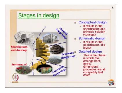
So, the next is stages in design. So, obviously, you need to know what are the different stages and what is this design process all about. Design phase is generally termed as an evolutionary process. You start with the customer requirements or demands and at the end of your whole design phase you are just generating some 500 - 600 drawings and along with a set of specifications. So, what happens in between that many of the people are really not very clear.
