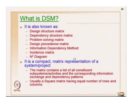
Now, let us move on to the technique, with the DSM how are we going to handle information-driven schedules. What is DSM? DSM is commonly known as design structure matrix because application is predominantly in the design phase. So, earlier when that tool came into existence when the technique came into existence it was named as design structure matrix only. Then, people started working with the construction phase also with for information sharing in construction phase for example; we have also
