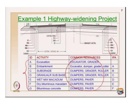
Now, let us take a highway widening a project this is example we have seen earlier for LOB or and so on. So, in this example what happens is this is a highway widening project. There is an existing carriageway here and this is primarily the carriageway which is proposed for widening and I have my embankment plan to be here and these are all the levels with which I have to fill my layers on the highways ok.
