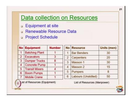
So, I have taken I am going to look at the activities only on the piers and pier cap, only the concreting activity alone equipment at site. So, these are the equipments I have a batching plant, 3 excavators, 8 dump trucks, 1 concrete pump, 4 transit mixers, 1 boom pump and 1 mobile crane I have in the site ok. Resource on manpower I have 30 bar benders, 12 20 carpenters, 30 mason first grade, 15 mason second grade and 8 pumpers and 50 unskilled workers I have in the particular case ok.
