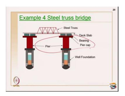
Now, let us take this another example in order to show the complexity with many resources coming in ok. This is a steal truss bridge ok. Primarily what happens, this is a simple steel truss. So, I have a steel truss here, this is my deck slab, these are my bearings I have a well foundations here, this is a pier cap and this is a pier. So, primarily I am going to look at pier and the pier cap activities only just concreting ok.
