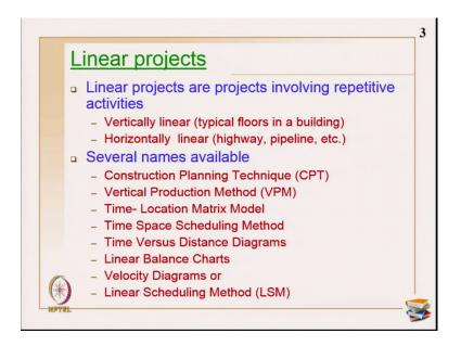
So Linear Projects; linear projects are the projects involving repetitive activities. It can be vertically or it can be horizontally repetitive in nature. Vertical repetitions primarily it is not linear. Vertical repetitions, For example, typical flows in a building. Horizontal repetitions can be highway projects pipeline projects and so on, ok.
