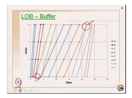
The next thing in LoB is the buffer. So, what happens in buffer and why should we introduce a buffer? Buffer is only for avoiding collision between the activities or we can say interference between the activities. Suppose if you do not introduce a buffer, you can see here the two activities are actually you know colliding with each other ok. There is something called collisions, ok. Primarily you need time for preparatory works or for setting up all your equipments and so on.
