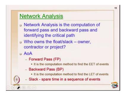
Now moving onto network analysis. So far we have seen network schedule, the terminology when you say network schedule is primarily representing your networks on to the with either in the AoA format or in the AoN format and the minute you say analysis, primarily you are going to do forward pass, backward pass, and critically you are going to find the critical activities in the path. So, network analysis is computation of forward pass and backward pass and identify the critical path.
