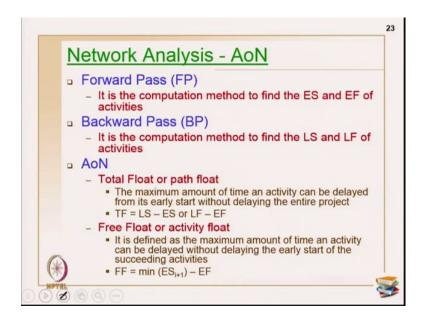
Now in the AoA method whether you are using or the AoN method the procedure for computation on analysis is same. First you have to do forward pass next backward pass and the flow calculations, in AoA we have slack calculations ok. That you should keep in mind.
