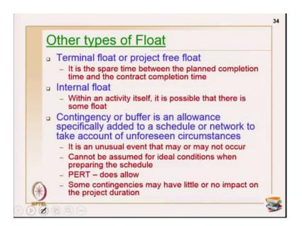
Then next type of floats is terminal float. So, terminal float is nothing but I have a whole project and there is really a different time for my planned completion and also for the contract completion, ok. In the earlier case I said if the contract completion or schedule pressure completion is little early you start getting a negatives on the floats, ok.
