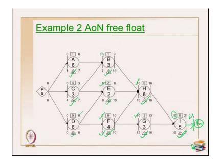
So, the next is free float. So, how do you calculate the free float? Free float for any activity is; so primarily the maximum of the early start of (Refer Time: 44:42) activity minus the early finish of the activity ok. For this particular activity I have only one successor and the early start is 6 minus the early finish is 6, so 6 minus 6 become 0 here. For this particular activity I have two successors and both the values happen to be the same, so 6 minus 3 is 3 for me.
