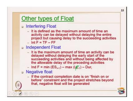
The next one is interfering float. These are all not much used, but there are other types also existing. So, it is defined as the maximum amount of time an activity can be delayed without delaying the entire project, but causing the delay to succeeding activities. So, this interfering float is generally TF minus FF, which implies total float minus free float, ok.
