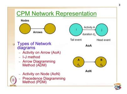
So, CPM network representation generally has two terminology: one is called nodes as you can see here; the nodes are generally in circle or in rectangles and the other one is called arrows. So, in the two types the way you represent the activities along the nodes or arrows we have the two methods.
