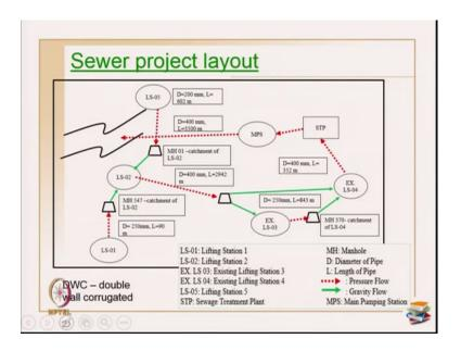
So, a little more on the layout. So, there are pressure flows, there are gravity flows in the area as well. So, you will have location of manholes like this, lifting stations are all here located at station 1, station 2, station 3, and there are manholes also based on the slope and gradients and the pressure on the flow of the sewer.
