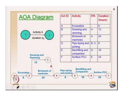
So, this is primarily the option which I have chosen and I have just represented the network, but there are other options also available and this dummy is introduced primarily to avoid the unique numbering of activities between the activity B and activity C. So, that is all on the AoA diagram.
