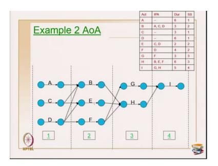
So, the same table I have shown it on the top for you to really correlate and understand. So, primarily the first sequence step, second sequence step, third sequence step and fourth sequence steps are given here. So, I have arranged my activities accordingly. This is activity on arrow diagram.
