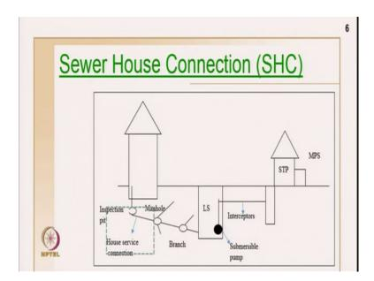
Now, let us take an example in order to really understand how to represent a AoA diagram and the analysis later on. So, first example primarily is a sewer house
