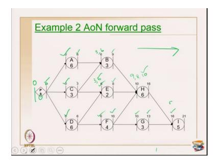
Now, first forward pass, as I told you earlier so primarily you have to put two lines close to each other and forward pass is primarily again from left to right, calculation of early start and early finish of all the activities ok. Project starts, so starting at 0 and the activity
