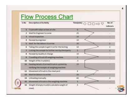
So, we used a simple diagram called flow process chart to measure all those. So, flow process chart. This is the flow process chart. These are all planning techniques as part of your work study which I will cover up at the end of the lecture on other scheduling techniques. I will give a small introduction to this. But I will just explain how to read this table first.
