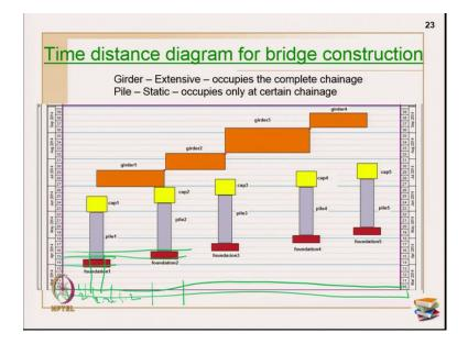
Now, let us move on in to see the time-chainage representations on TILOS. This is again a TILOS snapshot only on the same project, where in I have raised a bridge also to continue with my highway construction ok. So, these are all girders here; the girders are primarily the extensive activities which are shown like blocks and they occupy the complete chainage ok, almost most of the chainage ok.
